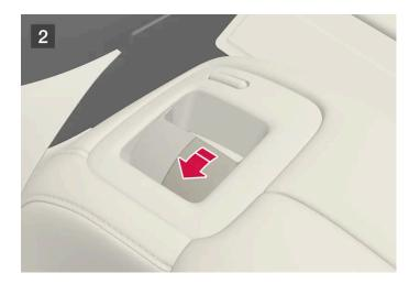
For cars without electronic folding, the outer head restraints are folded manually using the inner control on the upper side of the seat; see figure 2.
