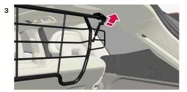
Position the safety grille's brackets on the roof mountings.
