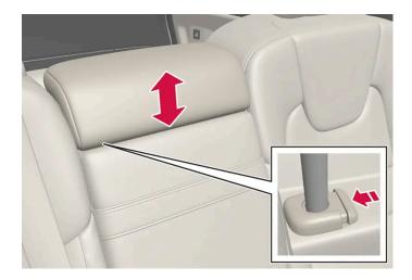
To lower the head restraint, the button (see illustration) must be depressed while the restraint is carefully moved down.
