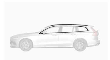
Parts that should be washed using a cleaning agent with a pH value between 3.5 and 11.5.
