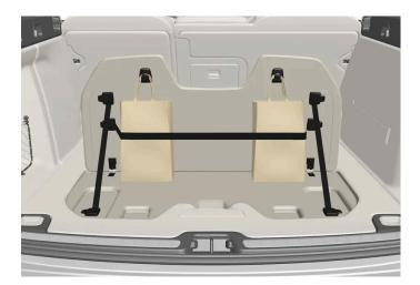
There are two bag hooks and an elastic strap<sup>[1]</sup> in the cover, which is part of the floor hatch in the cargo area. The strap can be fitted in four different positions.
