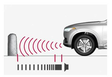
The warning signal has a constant acoustic signal at less than approx. 30 cm (1 foot) from an obstacle.
