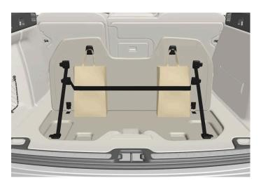
There are two bag hooks and an elastic strap<sup>[1]</sup> in the cover, which is part of the floor hatch in the cargo area. The strap can be fitted in four different positions.
