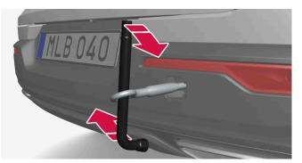
Screw the eye in firmly. For example, thread through the wheel bolt wrench\* and use it as a lever.
