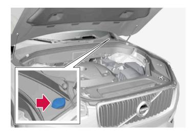
Washer fluid is filled into the reservoir with the blue cap. The reservoir is used for windscreen washer, rear window washer and headlamp washers\*.
