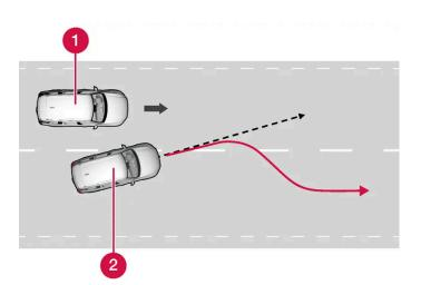
The function can assist by steering the car back to its own lane.
