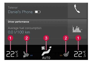
1 Temperature controls for driver and passenger side.
