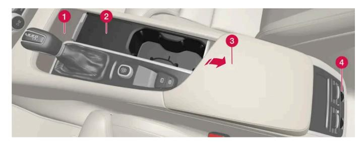
$\bigcirc$  Storage compartment hatch \* and 12 V socket<sup>[1]</sup>. The hatch is opened/closed with a push on the handle.
