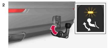
Lock the towbar by moving it back to its retracted position, where it is locked.
