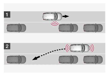
Principle for reversing into parallel parking.
