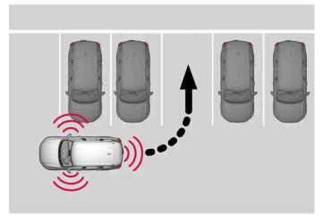
Principle for reversing into perpendicular parking.
