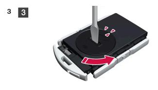
Turn the battery cover anticlockwise to OPEN position. Use a screwdriver or a coin, for example. Lift off the battery cover. If it is difficult to detach, you can prize it upward using a narrow tool.
