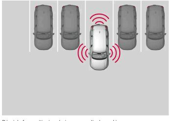
Principle for positioning during perpendicular parking.
