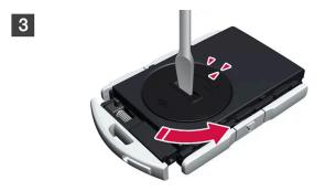
Turn the battery cover anticlockwise to OPEN position. Use a screwdriver or a coin, for example.
