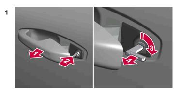
Pull out the front door's handle on the left-hand side of the car to its end position.<sup>[1]</sup>
