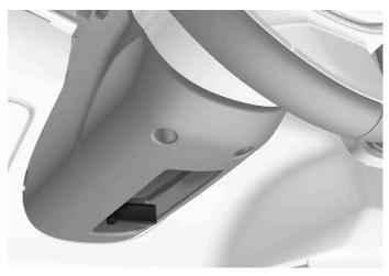
Lever for steering wheel adjustment.
