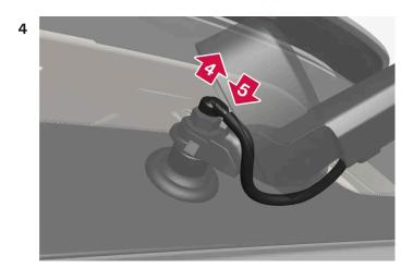
Loosen the washer hose from the bracket.
