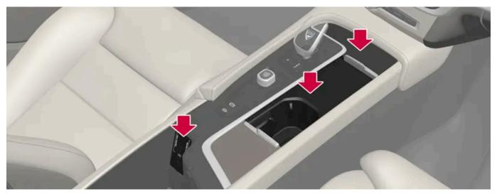
Storage spaces with cup holder, wireless phone charger  $\star$ , electrical socket, as well as USB ports in the tunnel console.
