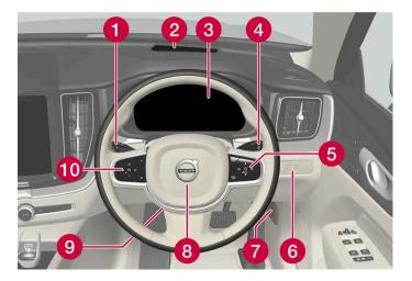
1 Position lamps, daytime running lights, dipped beam, main beam, direction indicators, front fog lamps/cornering lights\*, rear fog lamp, resetting the trip meter
