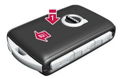
Turn the key and refit the front shell in the same way as for the rear.
