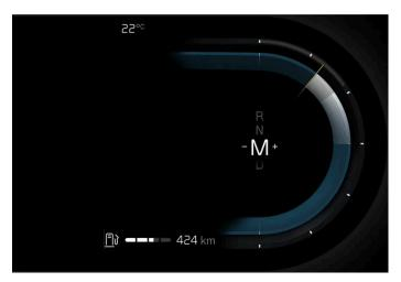
Gear shift indicator in the driver display.
