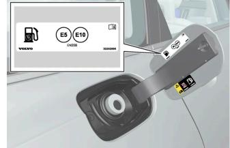
Choose fuel that is approved for use in the car in accordance with the identifier [1] on the inside of the fuel filler flap. See information on approved fuels and the identifier in the sections on "Petrol" and "Diesel" respectively.
