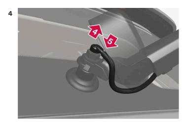
Loosen the washer hose from the bracket.
