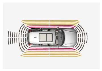
The warning signal pulses intensively at less than approx.  $25\ \text{cm}$  (0.8 foot) from an obstacle.
