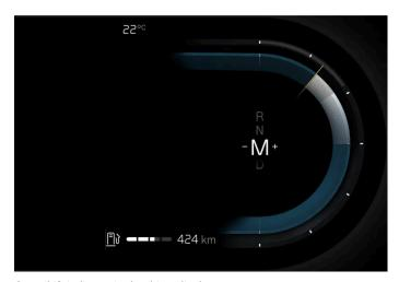
Gear shift indicator in the driver display.
