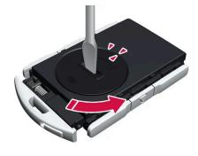
Turn the battery cover anticlockwise to OPEN position. Use a screwdriver or a coin, for example.
