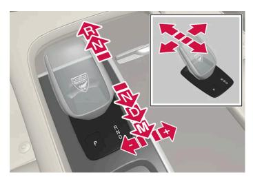
Overview of gear lever and gear positions.
