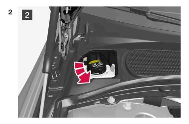
Screw off the cap and top up with coolant if necessary. The coolant level must lie between the  $\mbox{MIN}$  and  $\mbox{MAX}$  marks on the expansion tank.
