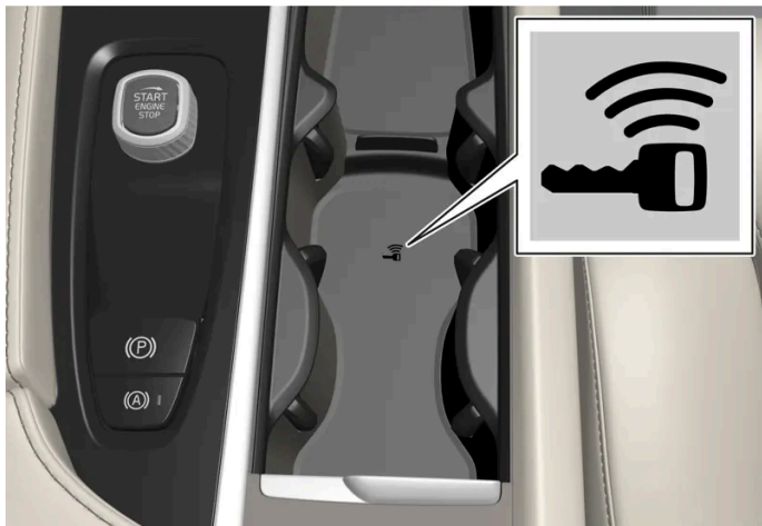
Backup reader's location in the tunnel console.
