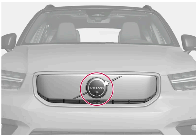
Location of front radar unit
