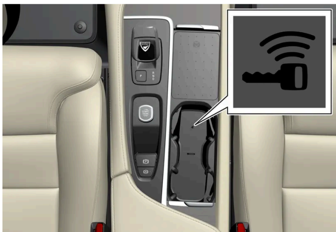
Backup reader's location in the tunnel console.
