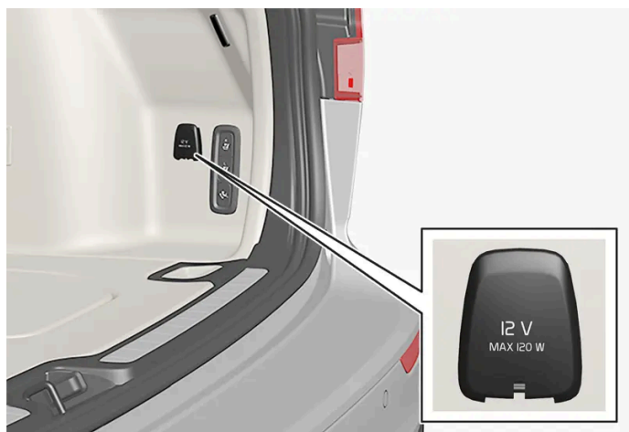
12 V electrical socket in cargo area*.
