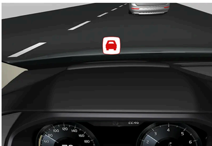
Symbol for collision warning on the windscreen
