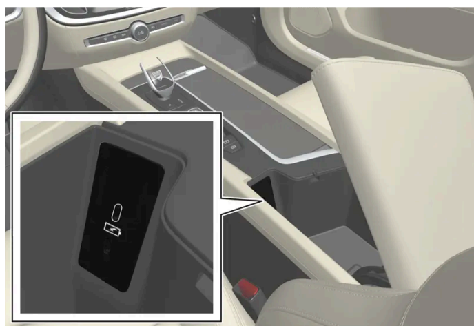
USB ports (type C), front seat.
