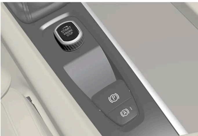
Start knob in the tunnel console.
