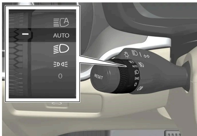
Stalk switch rotating ring in AUTO position.
