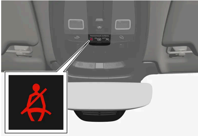
Visual reminder in the roof console.
