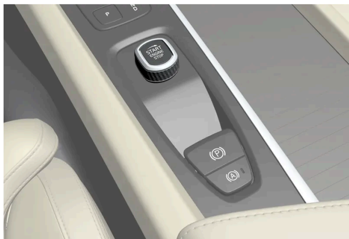
Start knob in the tunnel console.
