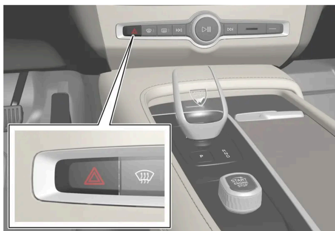
Button for hazard warning flashers.
