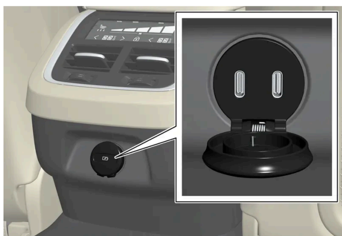
USB ports (type C) in the tunnel console, rear seat.
