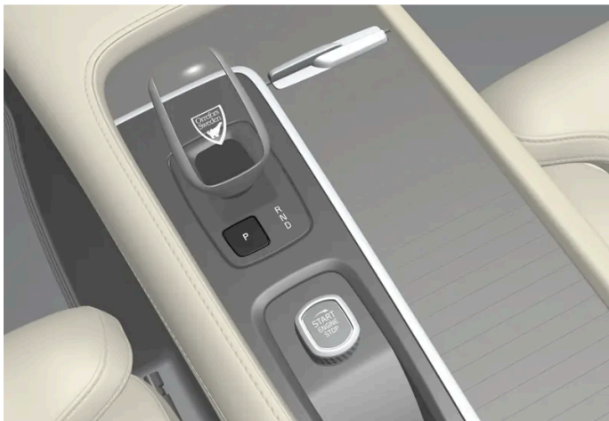
Overview of gear lever and position P.
