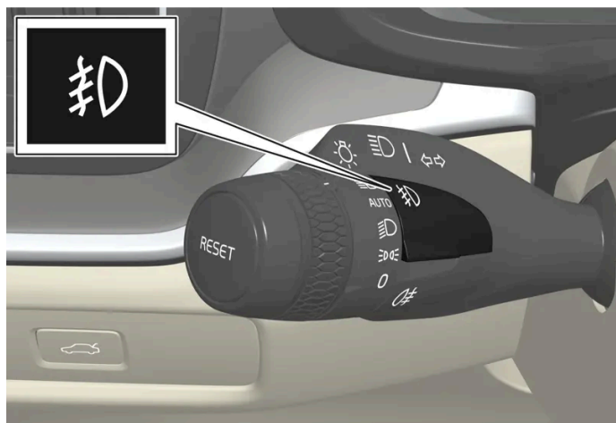
Button for front fog lamps.
