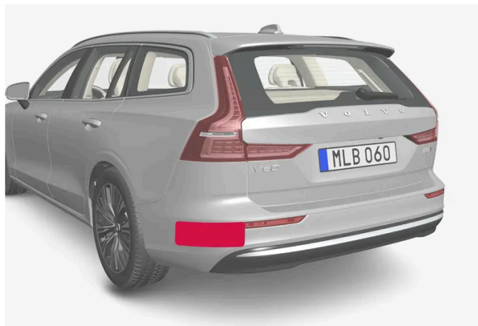
Location of rear radar units
