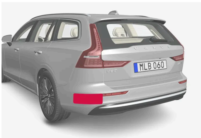
Location of rear radar units
