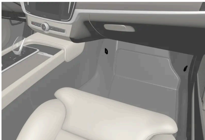
Mounting point locations in the front seat.
