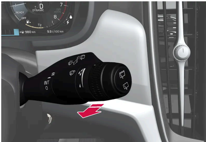
Washing function, right-hand stalk switch.
