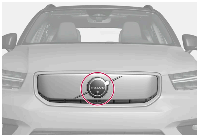
Location of front radar unit
