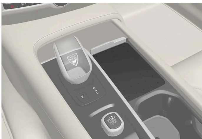
Wireless charger in the tunnel console.
