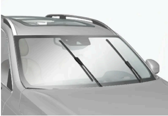
Wiper blades in service position.
