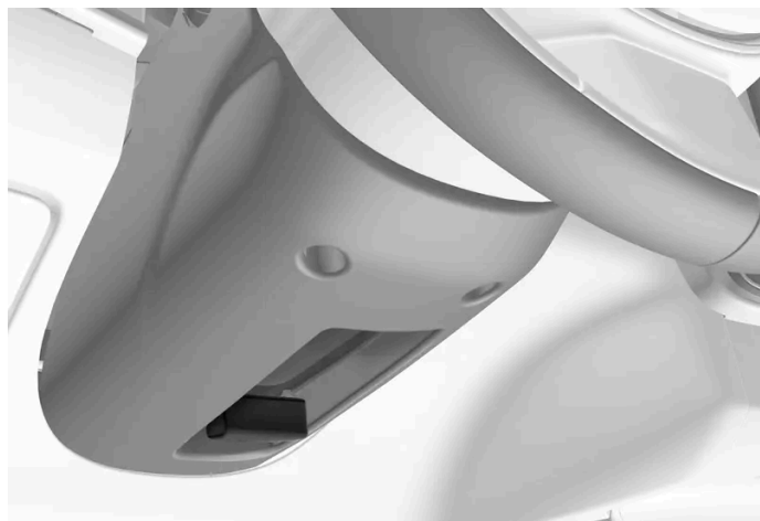
Lever for steering wheel adjustment.
