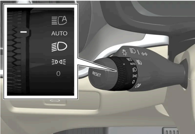
Rotating ring in the left-hand stalk switch.
