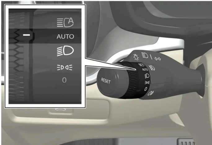
Stalk switch rotating ring in AUTO position.
