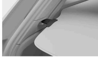
Lift and pull the end of the load cover screen by the handle to unlock it. This allows the load screen to retract.
