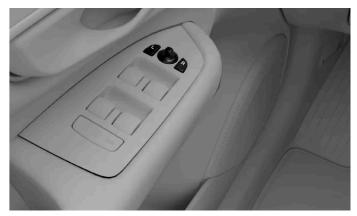
Controls for adjusting the wing mirrors
