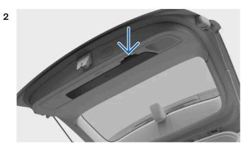
The warning triangle is located on the inside of the boot hatch. Pull the handle to open it.
