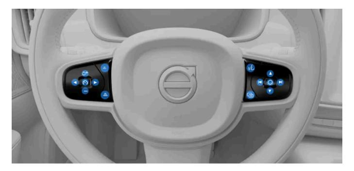
The buttons on your steering wheel's left-hand side control driver support features.
