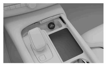
The 12 V socket in the tunnel console
