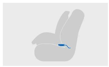
Child restraint installed using ISOFIX
