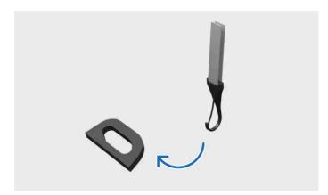
Fastening tether to lower tether anchorage point
