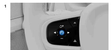
When it's safe to do so, press the Pilot Assist button (5) on the steering wheel.
