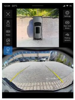
The parking view can display two views at the same time. The image shows an example of what it can look like after selecting the rear camera view, which is shown in the bottom half of the centre display. The top half of the display shows an overview of your car's surroundings.
