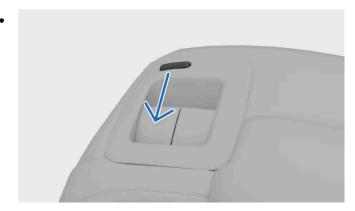
Pull the handle on the seat backrest. A red indicator near the backrest lock indicates that the backrest is no longer locked.
