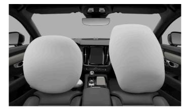
The driver side and the passenger side each have one front airbag. The driver side airbag is packed inside the steering wheel and the passenger side airbag is packed behind a panel above the glove box.
