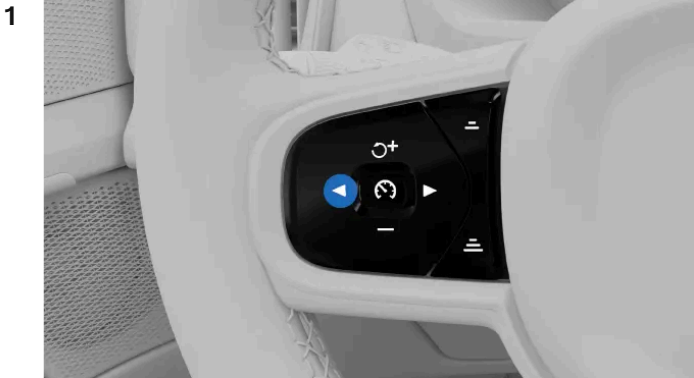
Press the disable ISA button ◀ on the steering wheel.
