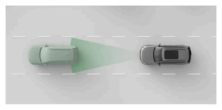
Adaptive cruise control<sup>[1]</sup> can support you with maintaining a set speed. When driving with adaptive cruise control active, you select a target speed. The car then manages acceleration and braking to meet that target while also adapting to surrounding traffic.
