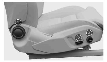
Overview of the seat adjustment controls on the side of the passenger seat.
