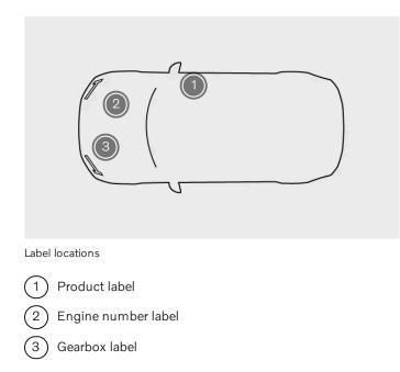
The product label is located on the right-hand door pillar and will be visible when the door is opened.
