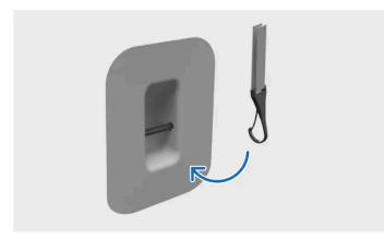
Fastening tether to top tether anchorage point
