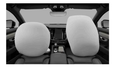
The driver side and the passenger side each have one front airbag. The driver side airbag is packed inside the steering wheel and the passenger side airbag is packed behind a panel above the glove box.
