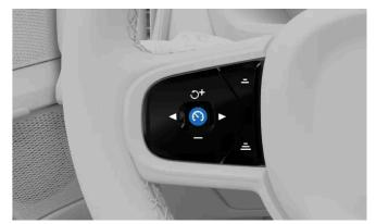
When it's safe to do so, press the adaptive cruise control button 🕥 on the steering wheel.
