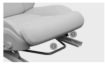
Overview of the seat adjustment controls beneath the passenger seat
