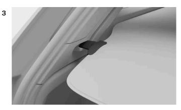
Guide the ends of the load cover into the locked position in the grooves.
