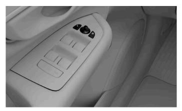
Controls for adjusting the wing mirrors
