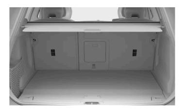
The top tether anchorage point locations for the rear seats are indicated by the top tether symbol.
