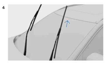
Press the button on the wiper arm and remove the wiper blade by pulling it upwards.
