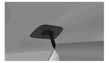
Fasten the lower corners of the net to the outer tether points behind the seats. 3
