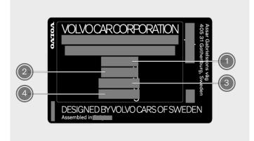
The label is located on the right-hand door pillar and will be visible when the door is opened.
