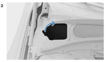
Open the panel hatch in the upper-left corner of the engine compartment to access the coolant container.
