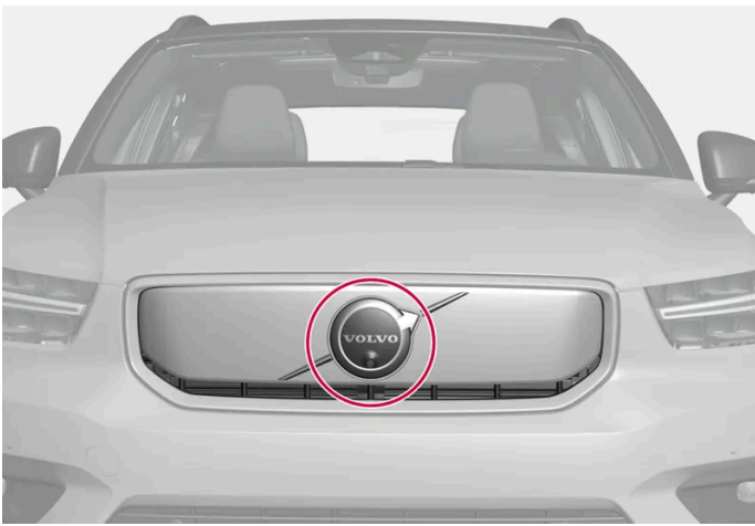
Location of front radar unit
