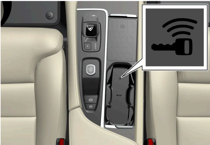
Backup reader's location in the tunnel console.
