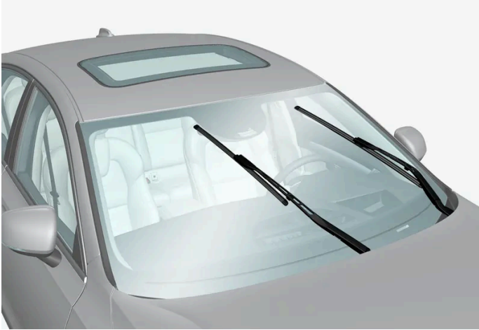
Wiper blades in service position.
