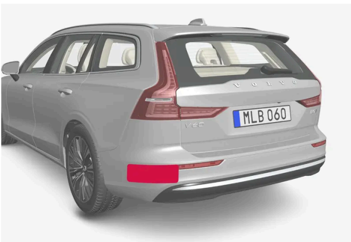
Location of rear radar units
