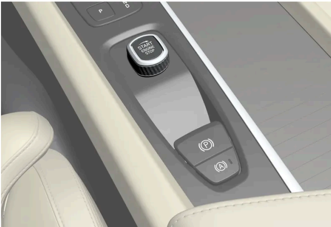
Start knob in the tunnel console.
