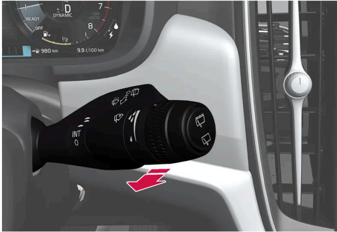
Washing function, right-hand stalk switch.
