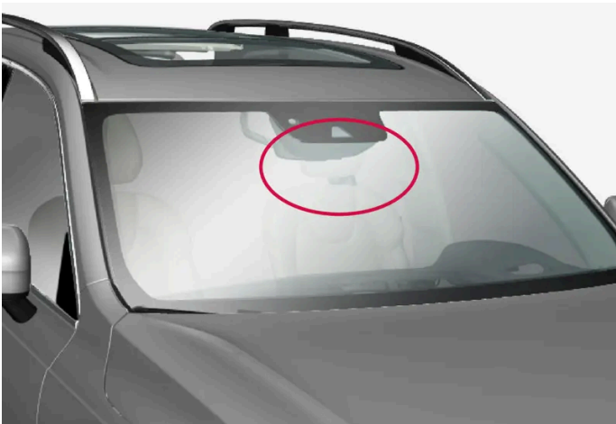
Location of the camera unit
