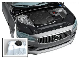
Coolant expansion tank, left-hand drive car.
