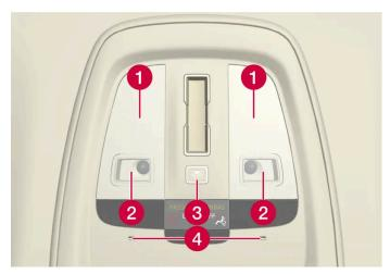
Lighting and controls in the roof console.
