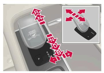
Overview of gear lever and gear positions.
