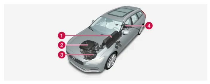
1 Hybrid battery - The function of the hybrid battery is to store energy. It receives energy when charging from the mains power circuit, during regenerative braking or from the high-voltage generator. It provides energy for electric operation as well as for temporarily operating the electric air conditioning during the preconditioning of the passenger compartment.
