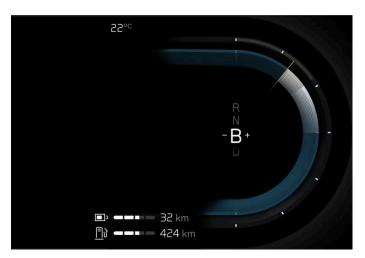
Gear shift indicator in the driver display.
