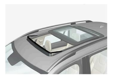
The panoramic roof has a wind deflector that is raised when the panoramic roof is in the open position.
