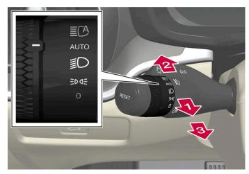
Steering wheel stalk switch with rotating ring.
