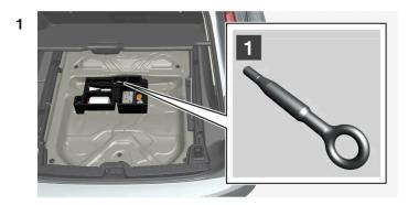
Take out the towing eye from the foam block under the floor in the cargo area<sup>[1]</sup>.
