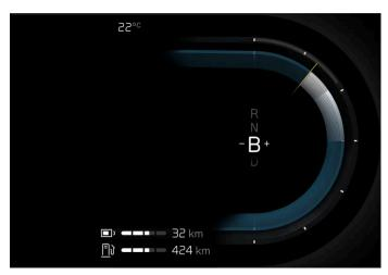
Gear shift indicator in the driver display.
