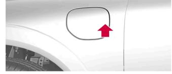
Press in the rear section of the cover to open the charging hatch<sup>[2]</sup>.
