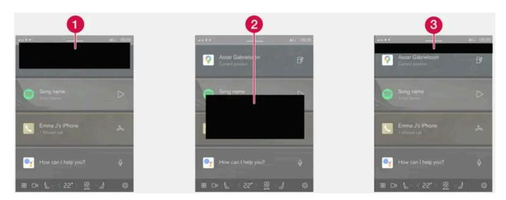
• Appears at the top of the centre display. Requires direct action and can have up to three buttons that allow the user to deal with the message. Dismiss by sweeping right or left, the message is then saved in notification view.
