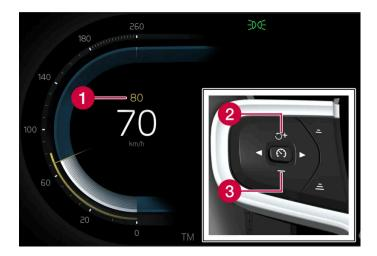
Stored speed + : Increases the stored speed - : Reduces stored speed
