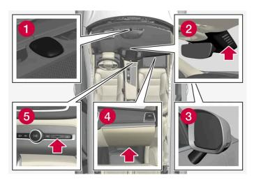
**1** Sun sensor - on the upper side of the instrument panel.
