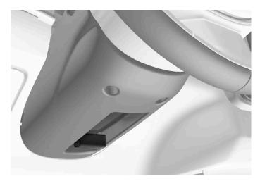
Lever for steering wheel adjustment.
