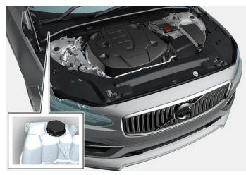
Coolant expansion tank, right-hand drive car.
