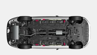
The car has outer lifting points for low level lifting, and inner lifting points for high level lifting, such as garage jack or lifting arms.
