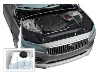
Coolant expansion tank, left-hand drive car.
