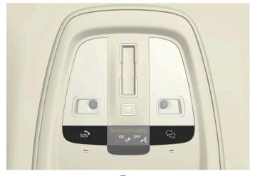
The functions are available via the  $\bigtriangledown$  and SOS buttons in the car's roof.
