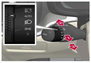
Steering wheel stalk switch with rotating ring.
