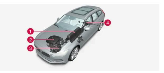
Hybrid battery - The function of the hybrid battery is to store energy. It receives energy when charging from the mains power circuit, during regenerative braking or from the high-voltage generator. It provides energy for electric operation as well as for temporarily operating the electric air conditioning during the preconditioning of the passenger compartment.
