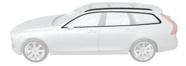
Parts that should be washed using a cleaning agent with a pH value between 3.5 and 11.5.
