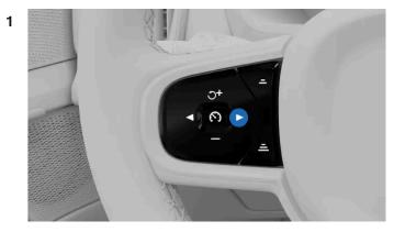
Press the switch button  $\blacktriangleright$  on the steering wheel.
