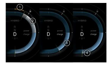
1) The car isn't able to draw its normal amount of power from the battery and the available power is reduced.
