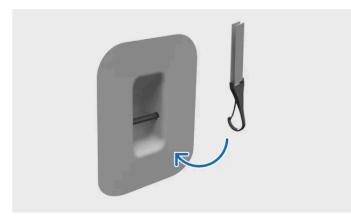
Fastening tether to top tether anchorage point
