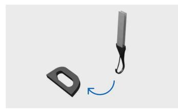
Fastening tether to lower tether anchorage point
