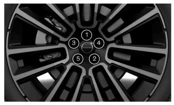
Tighten the wheel fasteners crosswise.
