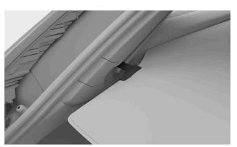
Lift and pull the end of the load cover screen by the handle to unlock it. This allows the load screen to retract.
