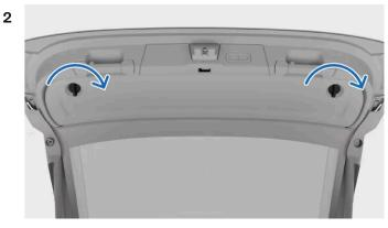
The warning triangle is located on the inside of the boot hatch. Open the compartment by turning the handles so that they are vertical and then pulling it.
