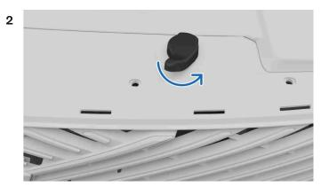
Locate the second lever below the front edge of the bonnet and rotate it anticlockwise.
