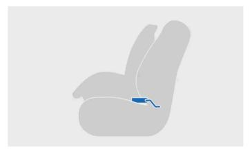
Child restraint installed using ISOFIX
