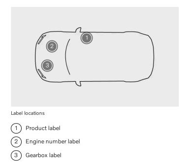
The product label is located on the right-hand door pillar and will be visible when the door is opened.
