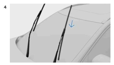
Make sure that the blade for the driver side is longer than the blade for the passenger side. Slide the wiper blade onto the wiper arm. Ensure that the pin on the wiper arm goes into the hole on the wiper blade. Push the blade into the wiper arm until you hear a click sound.
