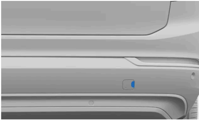
Rear towing eye fastening cover
