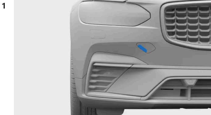
Front towing eye fastening cover
