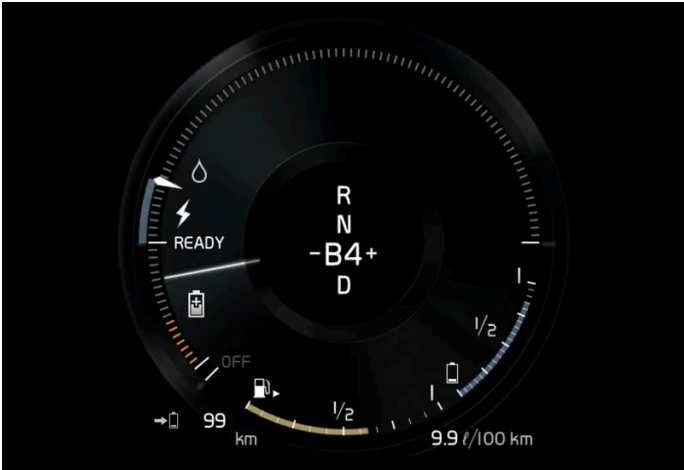
The driver display indicates charging during electric motor braking.
