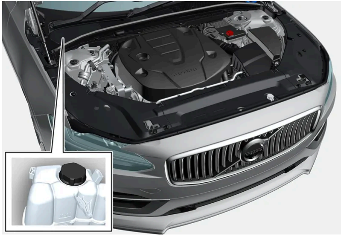
Coolant expansion tank, right-hand drive car
