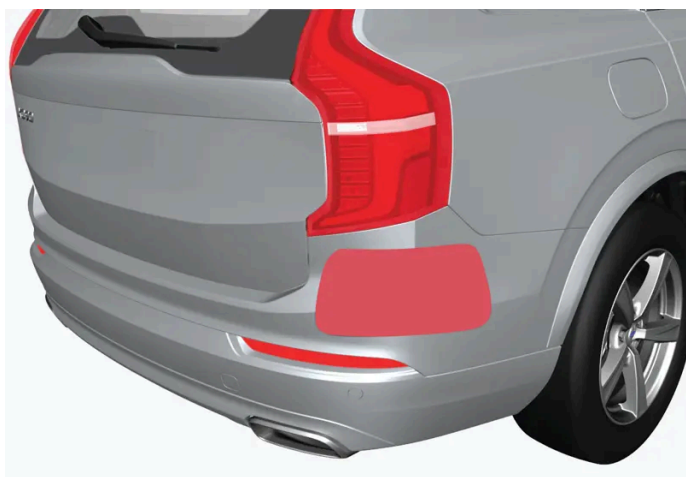
Location of rear radar units
