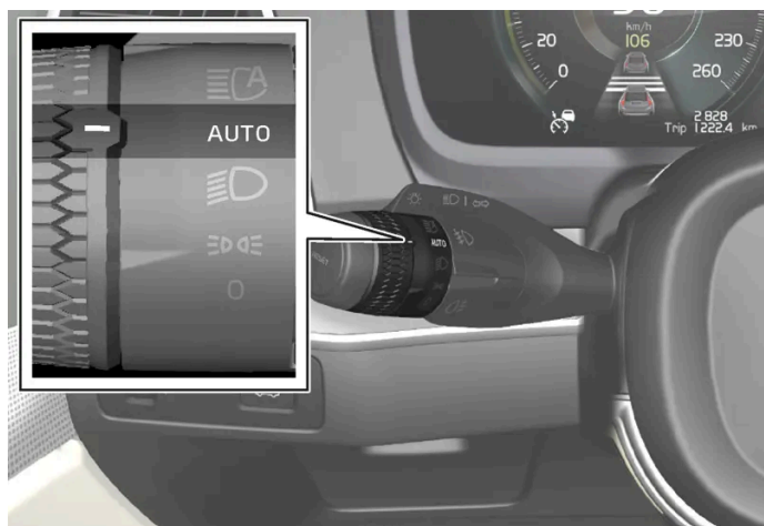
Stalk switch rotating ring in AUTO position.
