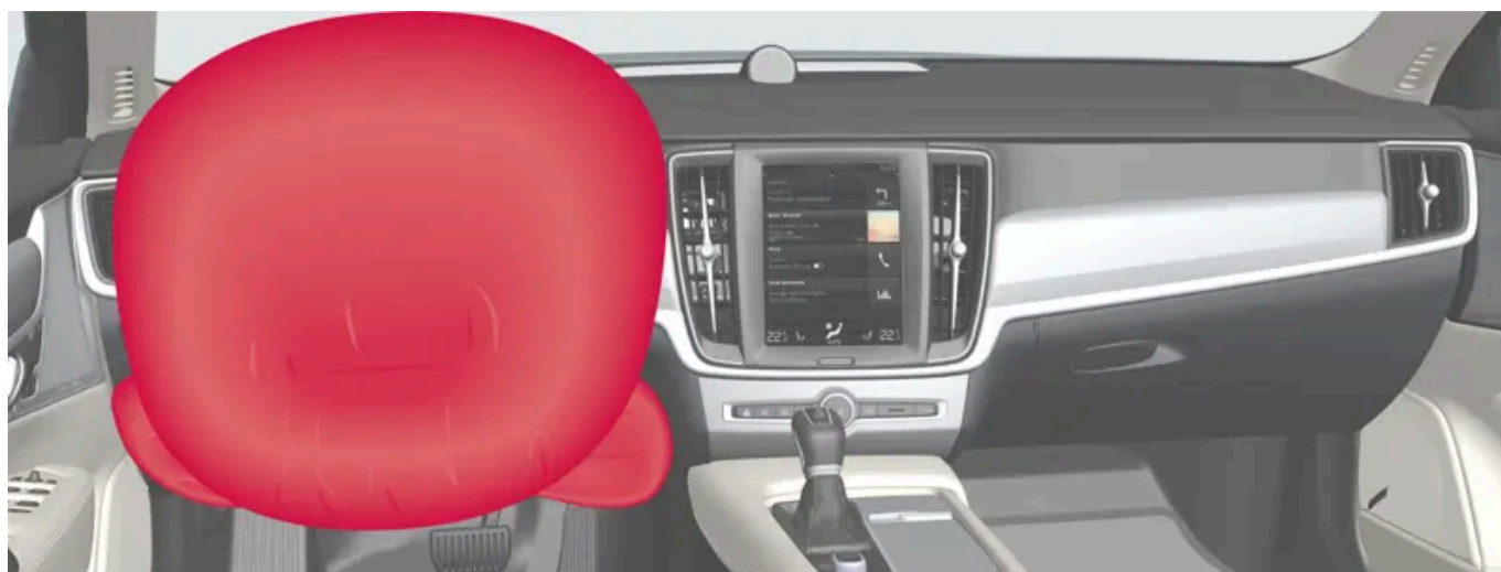
Steering wheel airbag and knee airbag [1] on the driver's side in the front seat.
