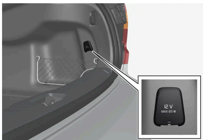
12 V electrical socket in cargo area*.
