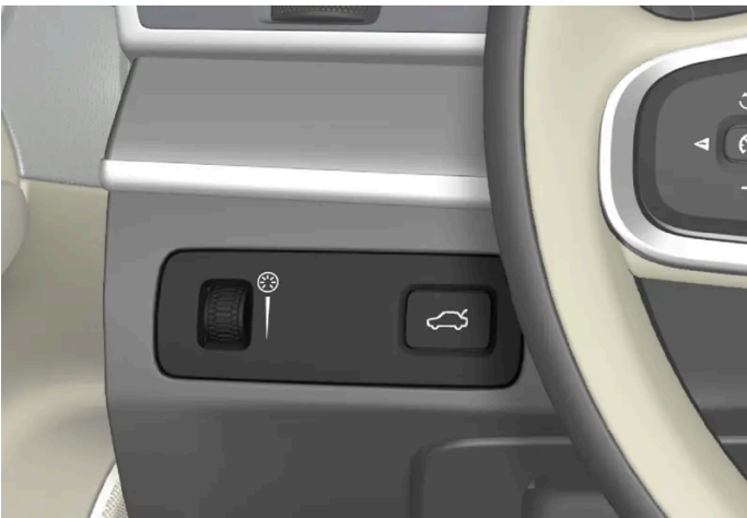
Thumbwheel (to left) for adjusting interior brightness.
