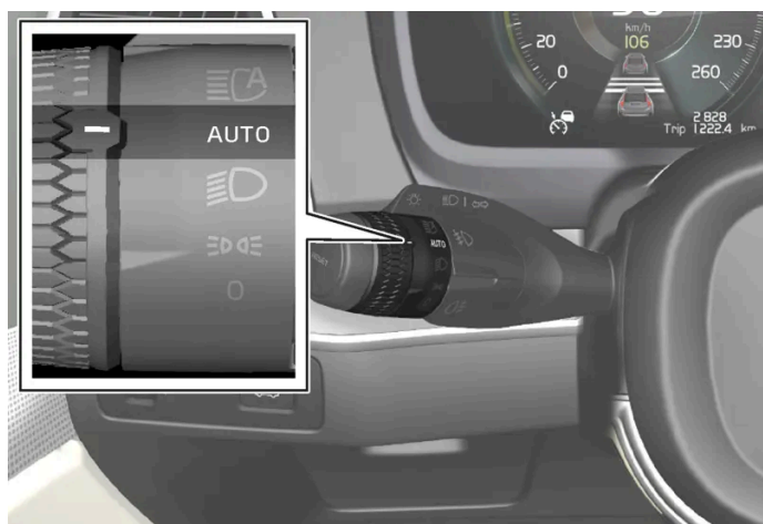
Stalk switch rotating ring in AUTO position.
