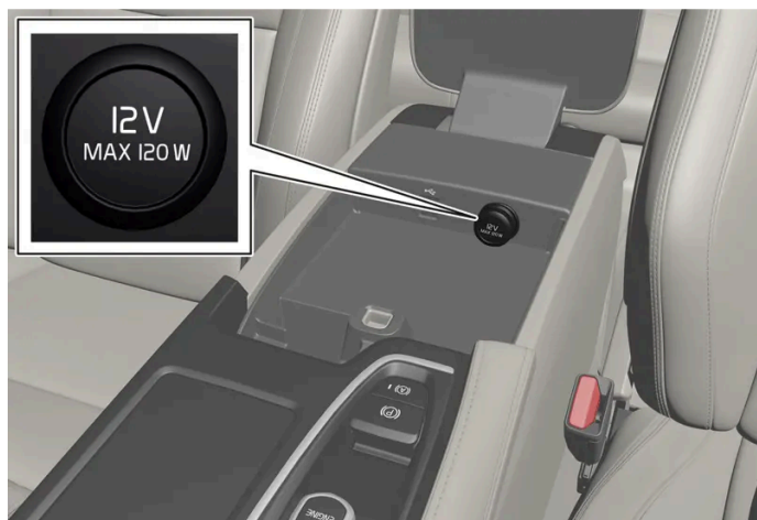
12 V electrical socket in tunnel console, front seat.
