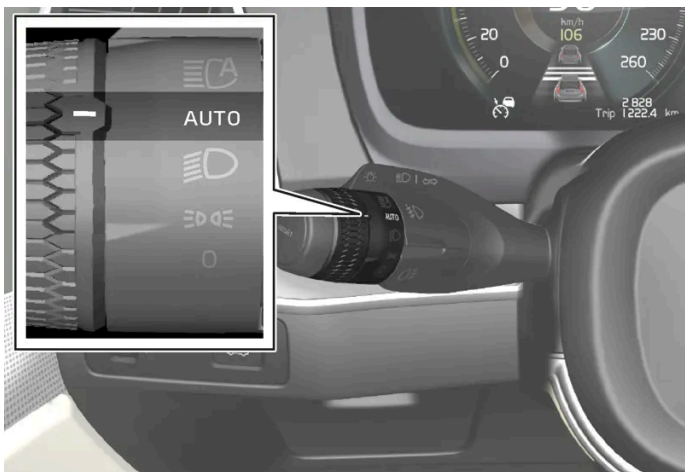
Stalk switch rotating ring in AUTO position.
