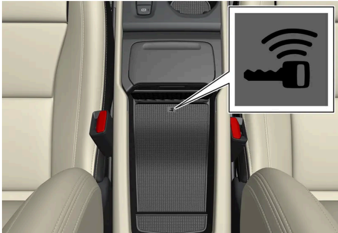
Backup reader's location in the tunnel console.
