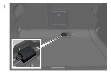
Fit a personal SIM card into the holder under the cargo area floor.
