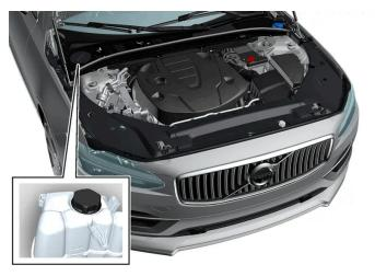
Coolant expansion tank, left-hand drive car
