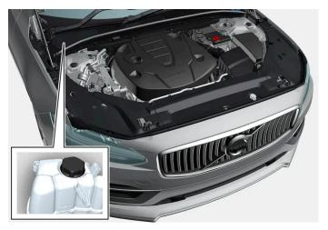
Coolant expansion tank, right-hand drive car
