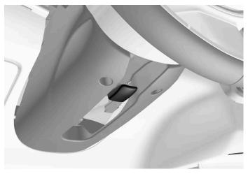
Lever for steering wheel adjustment.
