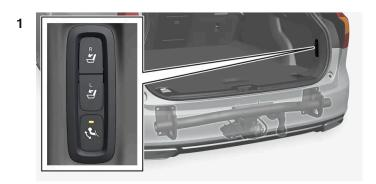
Open the tailgate. A button for extending/retracting the towbar is located on the right-hand side at the rear of the cargo area. An indicator lamp in the button must illuminate with a constant orange glow for the extension function to be active.
