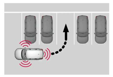
Principle for reversing into perpendicular parking.
