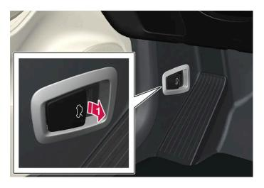
Pull the handle on the left of the brake pedal in order to release the bonnet from fully closed position.
