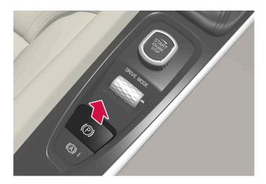
1 Pull the control upward.
