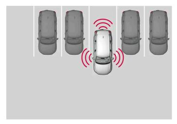
Principle for positioning during perpendicular parking.
