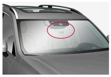
Location of front camera and radar unit
