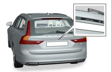
Rubberised pressure plate on the tailgate can only be used for unlocking.
