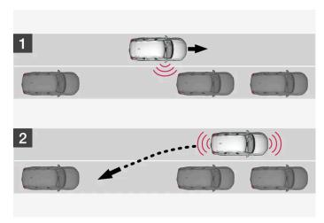
Principle for reversing into parallel parking.
