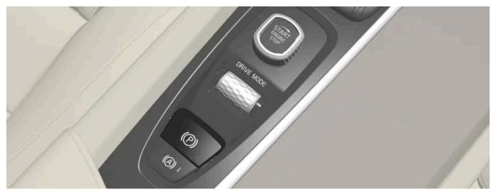
The control for the parking brake is located in the tunnel console between the seats.
