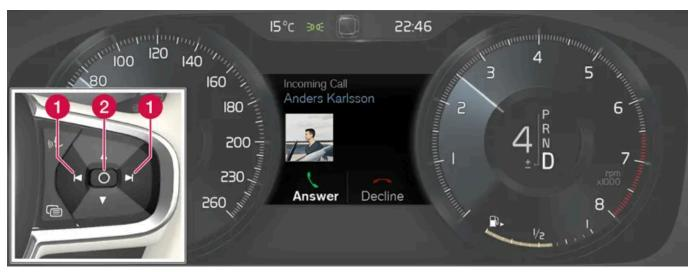
Examples of messages in the driver display [2] and the steering wheel's right-hand keypad. The figure is schematic - parts may vary depending on car model.
