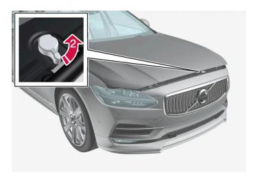
[2] Turn the handle under the bonnet anticlockwise to release the bonnet from the lock catches and lift the bonnet.
