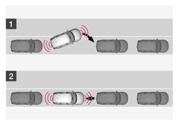
Principle for positioning during parallel parking.
