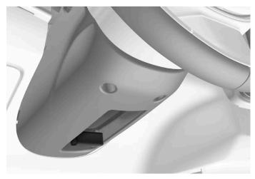
Lever for steering wheel adjustment.
