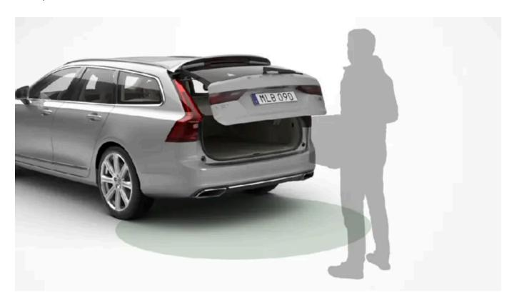
If the car is equipped with keyless locking and unlocking \* then you can unlock the tailgate with a foot movement.
