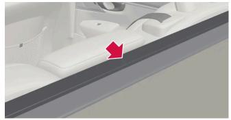
Fold the cargo cover's front panel forward to eliminate the space between the cargo cover and the rear seat's backrests.
