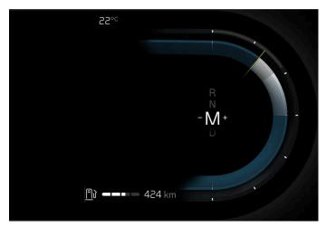
Gear shift indicator in the driver display.
