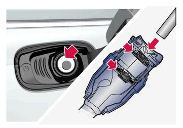
It is important to feed the pump nozzle past the filler pipe's two openable hatches before starting to fuel the car.
