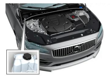
Coolant expansion tank, left-hand drive car.
