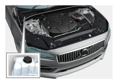
Coolant expansion tank, right-hand drive car.
