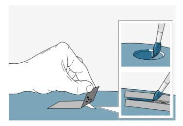
If the damage has not reached down to the metal, the touch-up paint can be applied directly after the surface has been cleaned.
