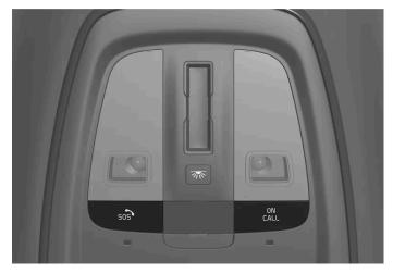
The functions are available via the  $\ensuremath{\mathsf{ON}}$  CALL and  $\ensuremath{\mathsf{SOS}}$  buttons in the car's roof.
