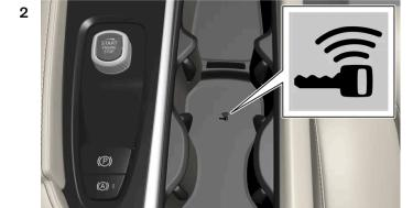
Place the key on the key symbol in the backup reader in the tunnel console's cup holder.
