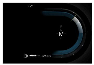
Gear shift indicator in the driver display.
