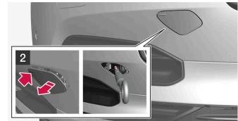
Front: Remove the cover - press on the marking with a finger.
