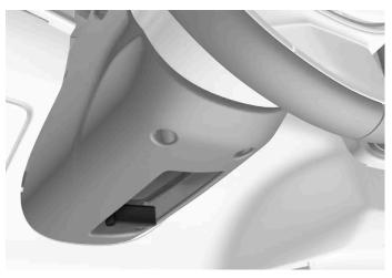
Lever for steering wheel adjustment.
