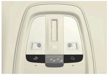
The functions are available via the  $\Re$  and SOS buttons in the car's roof.
