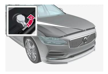
Turn the handle under the bonnet anticlockwise to release the catch and lift the bonnet.
