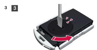
Turn the battery cover anticlockwise to OPEN position. Use a screwdriver or a coin, for example.
