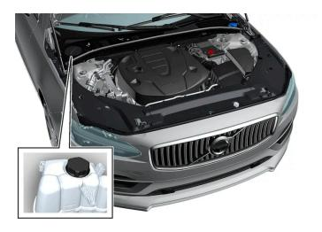
Coolant expansion tank, left-hand drive car.
