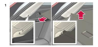
Grip the handle and pull out the cargo cover so that it slides over the side panels in the cargo area. Pull to the end position.
