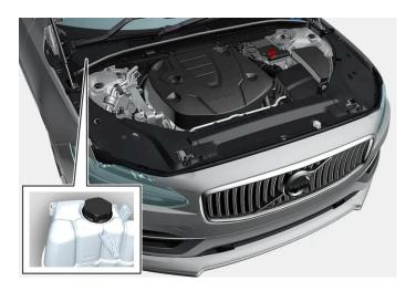
Coolant expansion tank, right-hand drive car.
