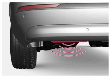
The sensor is located slightly to the left of the bumper.
