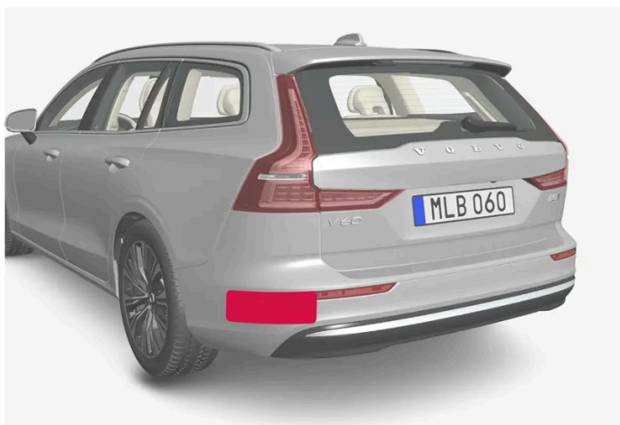
Location of rear radar units
