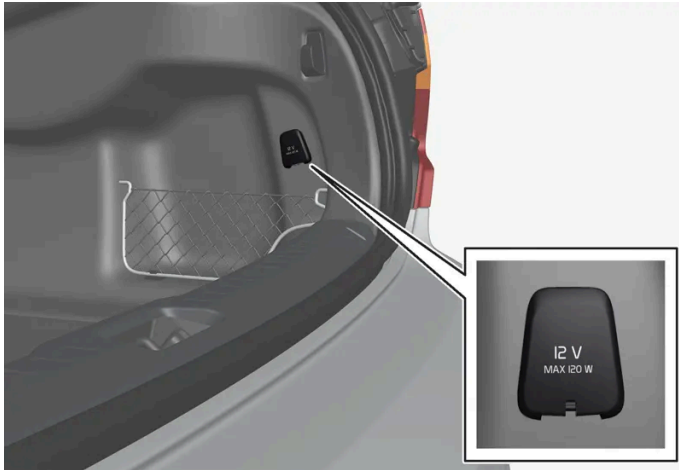
12 V electrical socket in cargo area*.
