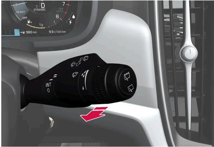
Washing function, right-hand stalk switch.
