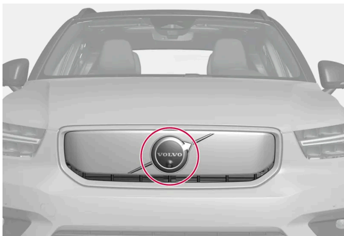
Location of front radar unit
