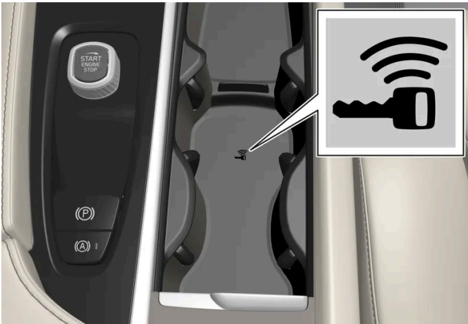
Backup reader's location in the tunnel console.
