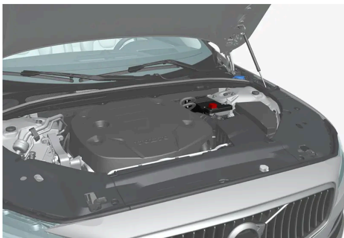
12 V support battery is located in the engine compartment.
