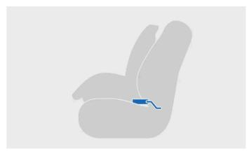
Child restraint installed using ISOFIX
