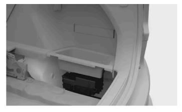
To access the fuse box you need to lift the panel on the right hand side of the boot.
