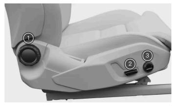
Overview of the seat adjustment controls on the side of the passenger seat.
