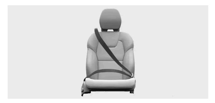
The seatbelt locks itself to act as a safety restraint under certain conditions, such as sudden and forceful pulling of the belt, if the car is driven aggressively and if the car is on a steep incline.
