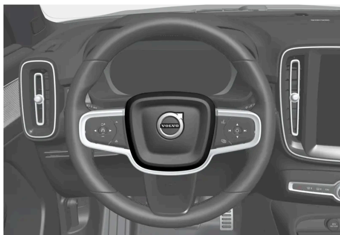
The horn is located in the centre of the steering wheel.
