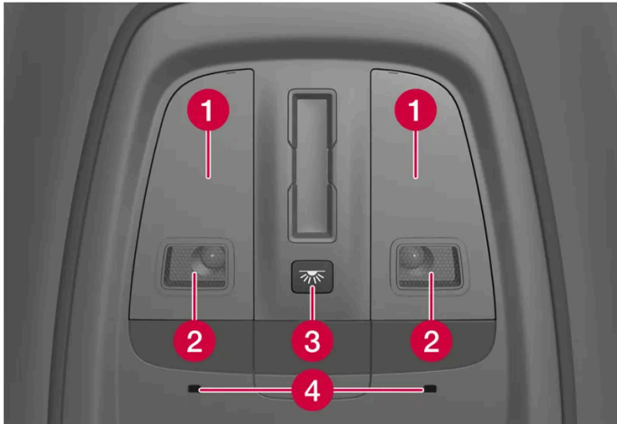
Lighting and controls in the roof console.
