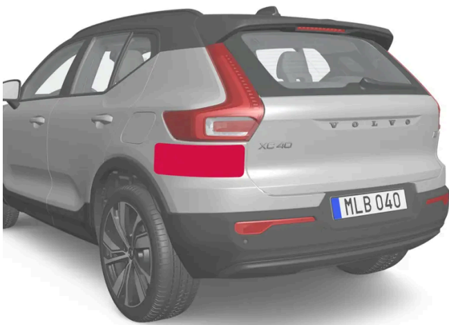
Location of rear radar units
