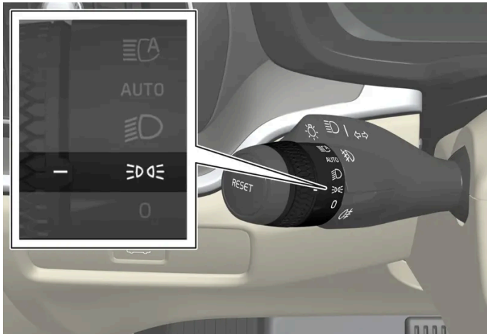
Stalk switch rotating ring in position lamps position.
