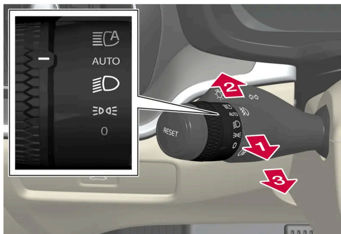
Steering wheel stalk switch with rotating ring.
