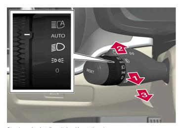
Steering wheel stalk switch with rotating ring.
