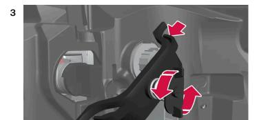
Unscrew and remove the spring bolt anticlockwise, press the clips into the sides and remove the supporting bridge. It is easiest to allow the screw to remain in the supporting bridge.
