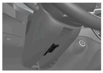
Lever for steering wheel adjustment.
