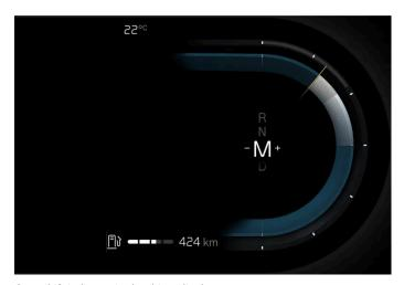
Gear shift indicator in the driver display.
