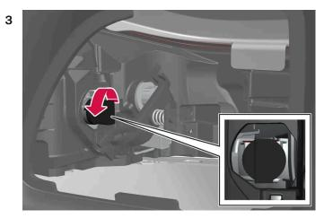
Undo the black bulb holder by turning it anticlockwise and pulling it out.
