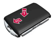
Refit the rear shell in reverse order to how it was removed. There is no logotype on the rear shell. Press in the shell until you hear a click, and then slide it the last few millimetres to its original position.
