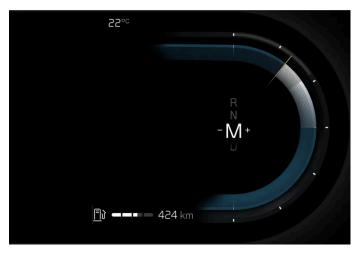
Gear shift indicator in the driver display.
