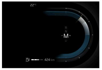
Gear shift indicator in the driver display.
