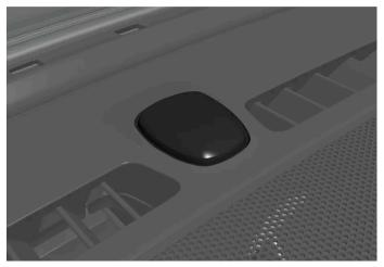
The indicator for locks and alarm is located in the centre of the instrument panel, close to the windscreen.
