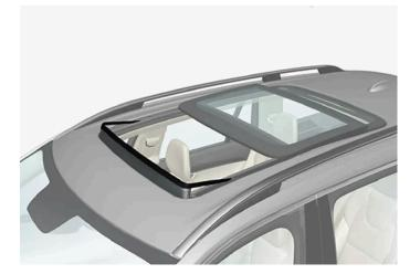
The panoramic roof has a wind deflector that is raised when the panoramic roof is in the open position.
