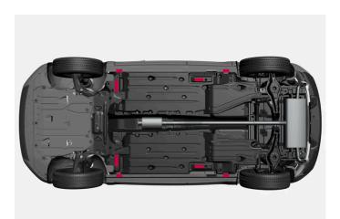
The car has outer lifting points for low level lifting, and inner lifting points for high level lifting, such as garage jack or lifting arms.
