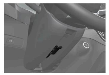
Lever for steering wheel adjustment.
