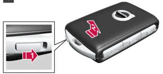
Slide the catch by the keyring bracket to the side, and slide the front shell away from the bracket.
