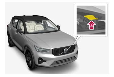
2 Move the handle under the bonnet upwards to release the catch and lift the bonnet.
