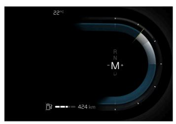
Gear shift indicator in the driver display.
