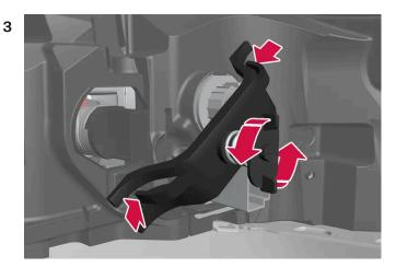
Unscrew and remove the spring bolt anticlockwise, press the clips into the sides and remove the supporting bridge. It is easiest to allow the screw to remain in the supporting bridge.
