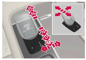
Overview of gear lever and gear positions.
