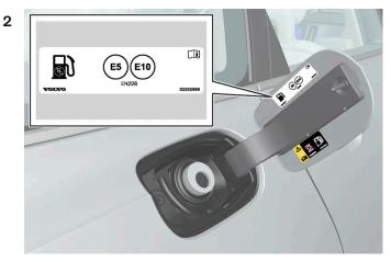
Choose fuel that is approved for use in the car in accordance with the identifier<sup>[1]</sup> on the inside of the fuel filler flap. See information on approved fuels and the identifier in the section on "Petrol".
