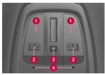
Lighting and controls in the roof console.
