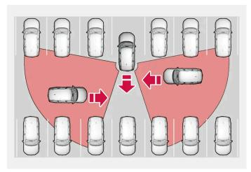
Examples of areas where the function can assist the driver to detect obstacles during reversing.
