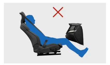
Do not tilt the backrest to a lying position. The seatbelt must remain tensioned against the shoulder.
