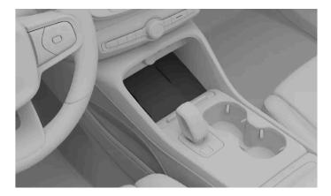
To use the wireless charger, your device should be certified to the Qi wireless charging standard. Also make sure that wireless charging is enabled on both the device [1] and on the charger itself. You can enable the charger in the centre display.
