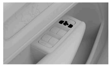
Controls for adjusting the wing mirrors
