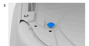
Locate the blue cap with the washer fluid symbol and open it.
