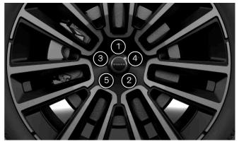
Tighten the wheel fasteners crosswise.
