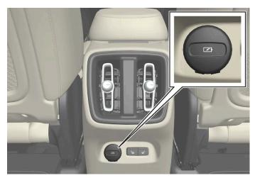
USB ports\* (type C) on rear of tunnel console for charging phones and tablets<sup>[1]</sup>, for example.
