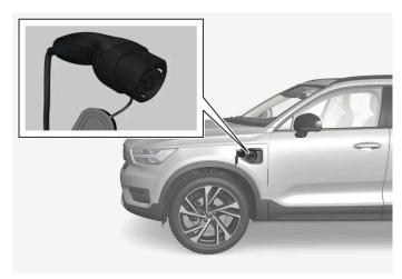
Charging cable handle and charging input socket.
