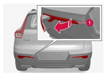
The rear fog light is only fitted on the driver's side.
