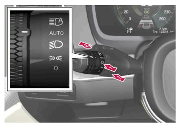
Steering wheel stalk switch with rotating ring.
