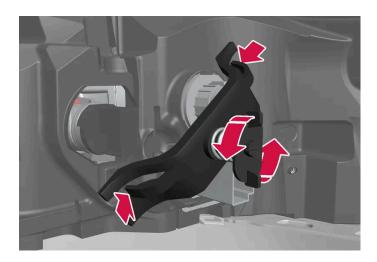
3. Unscrew and remove the spring bolt anticlockwise, press the clips into the sides and remove the supporting bridge. It is easiest to allow the screw to remain in the supporting bridge.
