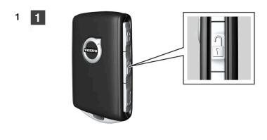
Unlock the car with the remote control key - charging is finished and the charging cable's locked handle releases/is unlocked.
