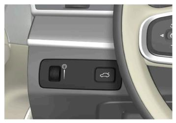
Thumbwheel (to left) for adjusting interior brightness.
