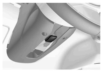
Lever for steering wheel adjustment.
