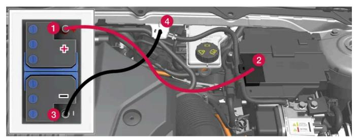
Charging point for jump-starting own car. There are two connection points under the cover. Only use the one closest to the passenger compartment.
