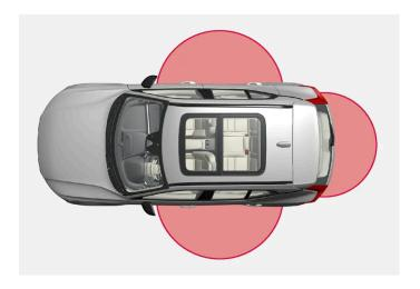
For keyless use, a remote control key or the button-less key (Key Tag) must be within a semicircular area with a radius of approx. 1.5 metres (5 feet) on both long sides and approx. 1 metre (3 feet) from the tailgate.
