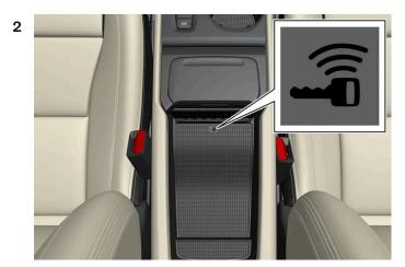
Place the remote control key on the key symbol in the backup reader in the tunnel console's storage compartment.
