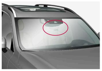
Location of front camera and radar unit
