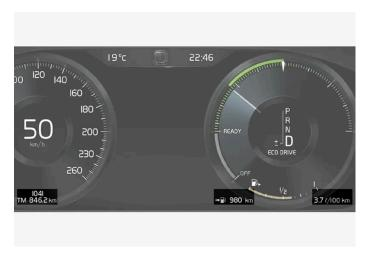
Examples of trip computer information in the driver display. The figure is schematic - parts may vary depending on car model.
