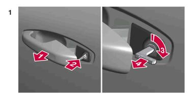
Pull out the front door handle on the left-hand side to its end position so that the lock cylinder becomes visible [1].
