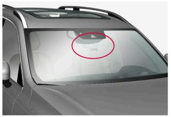
Location of front camera and radar unit
