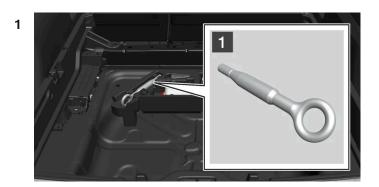
Take out the towing eye from the foam block under the floor in the cargo area.
