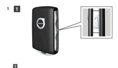
Unlock the car with the key - charging is finished and the charging cable's locked handle releases/is unlocked.
