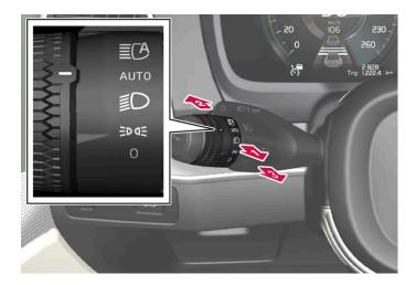
Steering wheel stalk switch with rotating ring.
