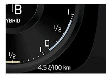
The energy in the hybrid battery is used for the electric motor, but also to cool or heat the car. The trip computer calculates an approximate distance for the energy left in the hybrid battery.
