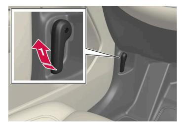
Pull the handle on the left of the brake pedal in order to release the bonnet from fully closed position.
