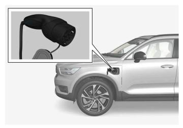
Charging cable handle and charging input socket.
