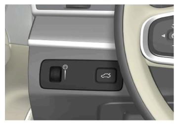
Thumbwheel (to left) for adjusting interior brightness.
