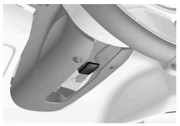
Lever for steering wheel adjustment.
