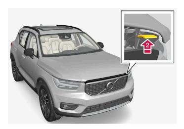
Move the handle under the bonnet upwards to release the bonnet from the lock catch and lift the bonnet.
