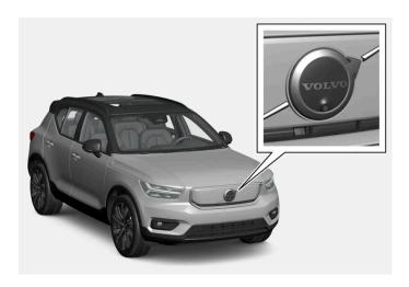
The front camera can be helpful on an exit road with limited visibility to the sides, e.g. when driving out of a garage. It is active at speeds up to 25 km/h (16 mph) - following which, the front camera is switched off.
