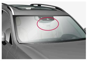
Location of front camera and radar unit
