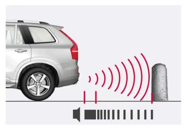
The warning signal has a constant tone at less than approx. 30 cm (1 foot) from an obstacle.
