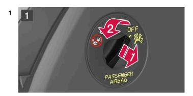
Pull the switch outward and turn from OFF to ON.
