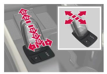
Overview of gear lever and gear positions.
