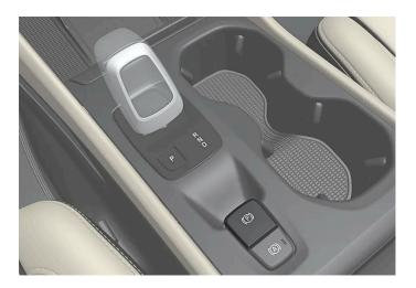
A faint electric motor noise can be heard when the electrically-operated parking brake is being applied. The noise can also be heard during the automatic function checking of the parking brake.
