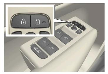
Lock buttons with indicator lamp in the front door.
