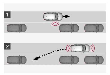
Principle for reversing into parallel parking.
