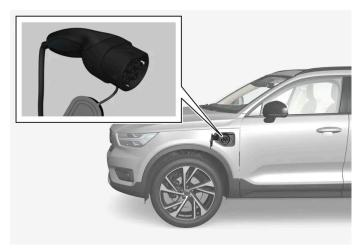
Charging cable handle and charging input socket.
