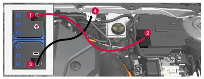
Charging points for jump starting own car. There are two connection points under the cover. Only use the one closest to the passenger compartment.
