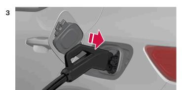
Grasp the charging cable with both hands and press the charging cable all the way into the car's charging input socket. The charging cable is automatically locked into the charging input socket after a couple of seconds. Ensure that the charging cable is properly locked so that charging can start.
