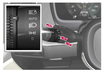
Steering wheel stalk switch with rotating ring.
