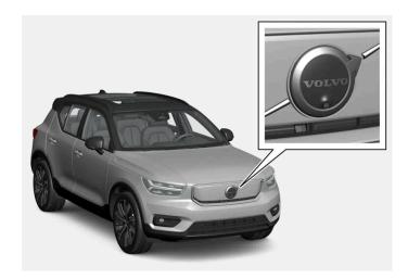
The front camera can be helpful on an exit road with limited visibility to the sides, e.g. when driving out of a garage. It is active at speeds up to 25 km/h (16 mph) - following which, the front camera is switched off.
