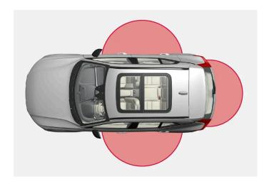
For keyless use, a remote control key or the button-less key (Key Tag) must be within a semicircular area with a radius of approx. 1.5 metres (5 feet) on both long sides and approx. 1 metre (3 feet) from the tailgate.
