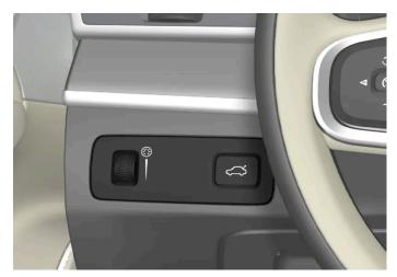
Thumbwheel (to left) for adjusting interior brightness.
