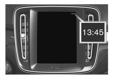
The clock is located at the top right of the centre display's status bar.
