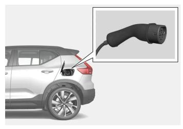
Charging cable handle and charging input socket.
