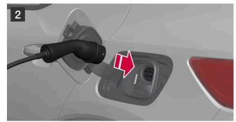
Open the charging hatch. Remove the charging handle's protective cover and make sure there are no objects in the charging input socket that may prevent charging.
