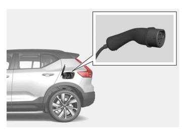
Charging cable handle and charging input socket.
