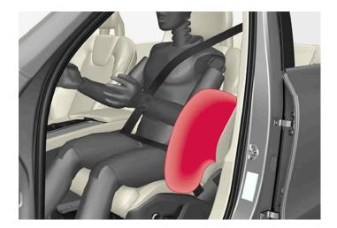
The side airbags are fitted in the outer backrest frames of the front seats and help to protect the driver and passengers in the
