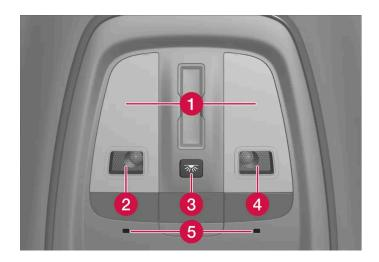
Lighting and controls in the roof console.
