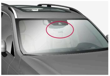
Location of front camera and radar unit
