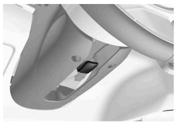
Lever for steering wheel adjustment.
