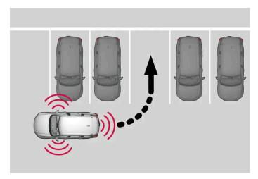
Principle for reversing into perpendicular parking.
