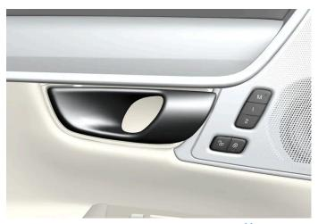
Opening handle for alternative unlocking in the side door [1].
