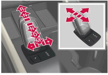
Overview of gear lever and gear positions.
