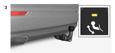
Move the towbar to its end position, where it is secured and locked in place - the indicator lamp illuminates with a constant orange glow.
