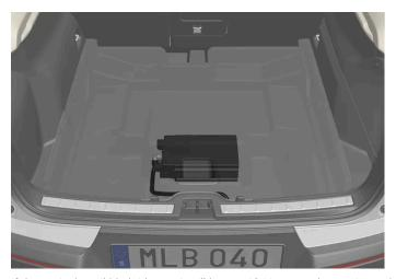
If the car is the mild hybrid type, it will have a 48 V support battery instead, which is located on the left of the cargo area. The 48 V support battery must only be handled by an authorised workshop.
