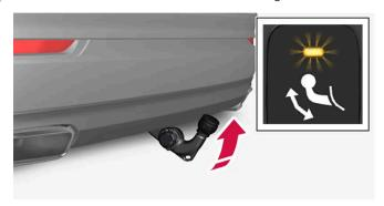
> The towbar extends out and down in an unlocked position - the indicator lamp flashes orange. The tow hook is ready to continue moving to the locked position.
