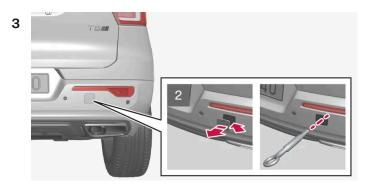
Rear: Remove the cover – Use a coin, key or similar to pry the lid out using the marking.
