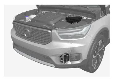
The 12 V support battery is located down in the engine compartment. The starter battery is also shown here (top).
