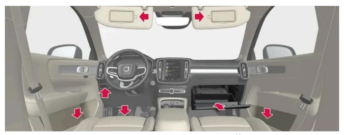
Storage compartment in door panel, card holder on left of steering wheel, storage under driver's seat<sup>[1]</sup>, sun visor and glovebox with extensible hook.
