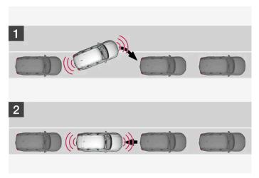
Principle for positioning during parallel parking.
