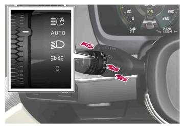
Steering wheel stalk switch with rotating ring.
