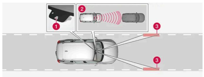
The camera and radar unit measures the distance to the vehicle ahead and detects side markings.
