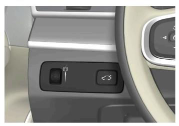
Thumbwheel (to left) for adjusting interior brightness.
