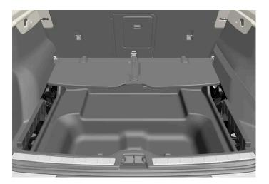
1 Lift the handle in the middle of the folding cargo area floor and fold it forwards.
