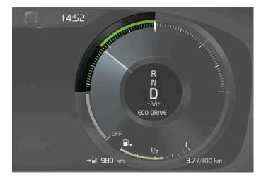
The ECO gauge indicates how fuel-efficient the driving is:
