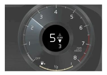
An up-arrow indicates a recommended change to a higher gear, and a down-arrow a recommended change to a lower gear.
