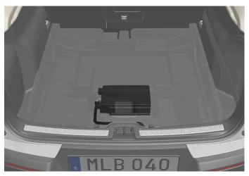
If the car is the mild hybrid type, it will have a 48 V support battery instead, located on the left-hand side of the cargo area. The battery must only be handled by an authorised workshop.
