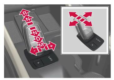
Overview of gear lever and gear positions.
