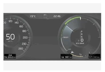
Examples of trip computer information in the driver display. The figure is schematic - parts may vary depending on car model.
