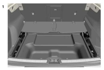
Fold up the folding cargo area floor forwards to be able to lower the parcel shelf downwards with the upper side turned down and the rear part facing forwards.
