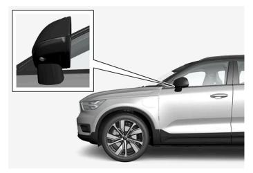
The side cameras are positioned in each door mirror.
