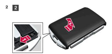
Slide the catch that was behind the front shell to the side, and slide the rear shell away from the key ring bracket.
