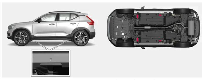
Arrows along the bottom edge of the side of the car mark where the jacking points/lifting points (marked in red) are located.
