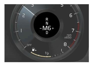
The gear shift indicator shows the current gear in the driver display and indicates recommended shifting to a higher gear by a flashing plus sign.
