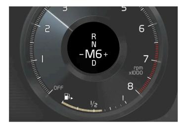
The gear shift indicator shows the current gear in the driver display and indicates recommended shifting to a higher gear by a flashing plus sign.
