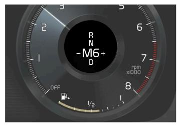
Overview of manual gear position in the driver display.
