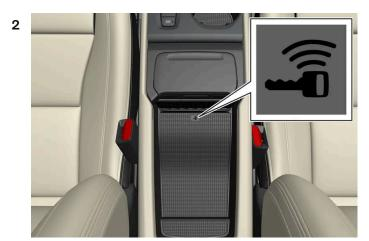
Place the key on the key symbol in the back-up reader in the tunnel console's storage compartment.
