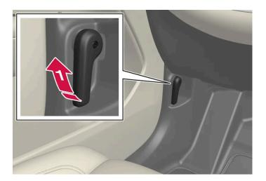
Pull the handle beside the pedals to release the bonnet from its fully closed position.
