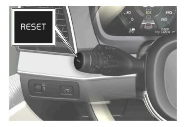
1 Reset all information in trip meter TM (i.e. mileage, average consumption, average speed and driving time) with a long press on the RESET button on the left-hand stalk switch.
