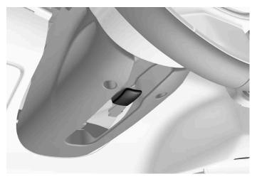
Lever for steering wheel adjustment.
