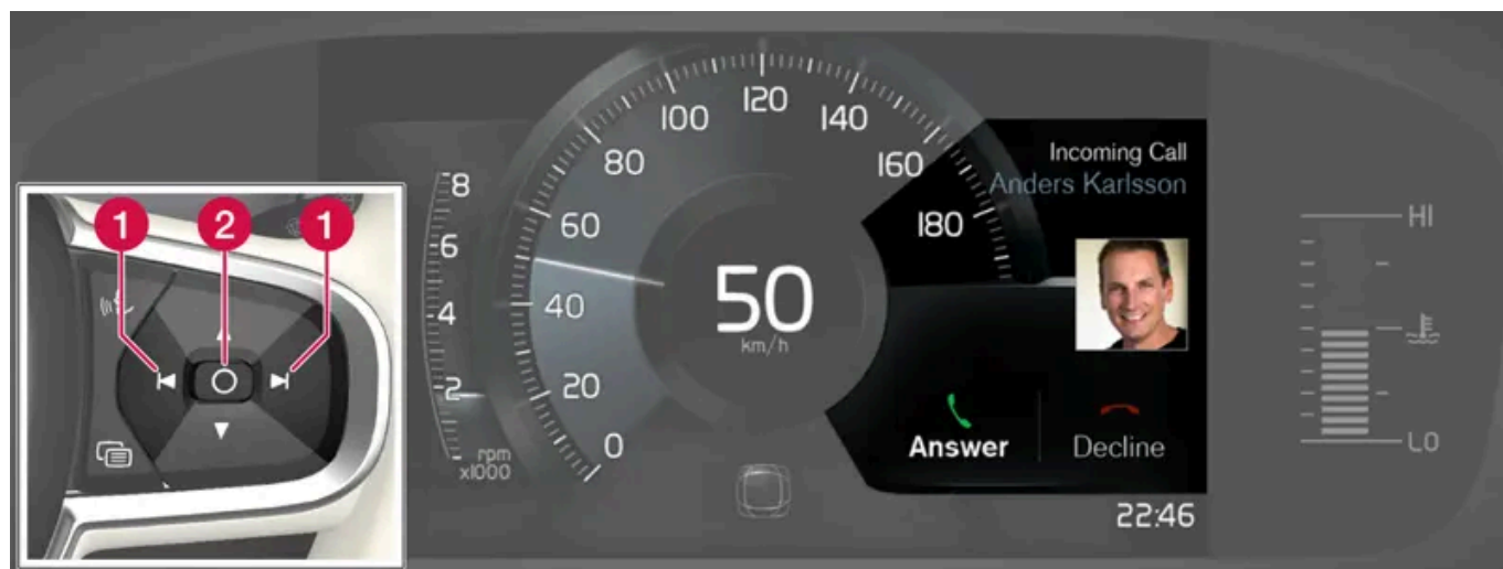
Examples of messages in the driver display [1] and the steering wheel's right-hand keypad. The figure is schematic - parts may vary depending on car model.
