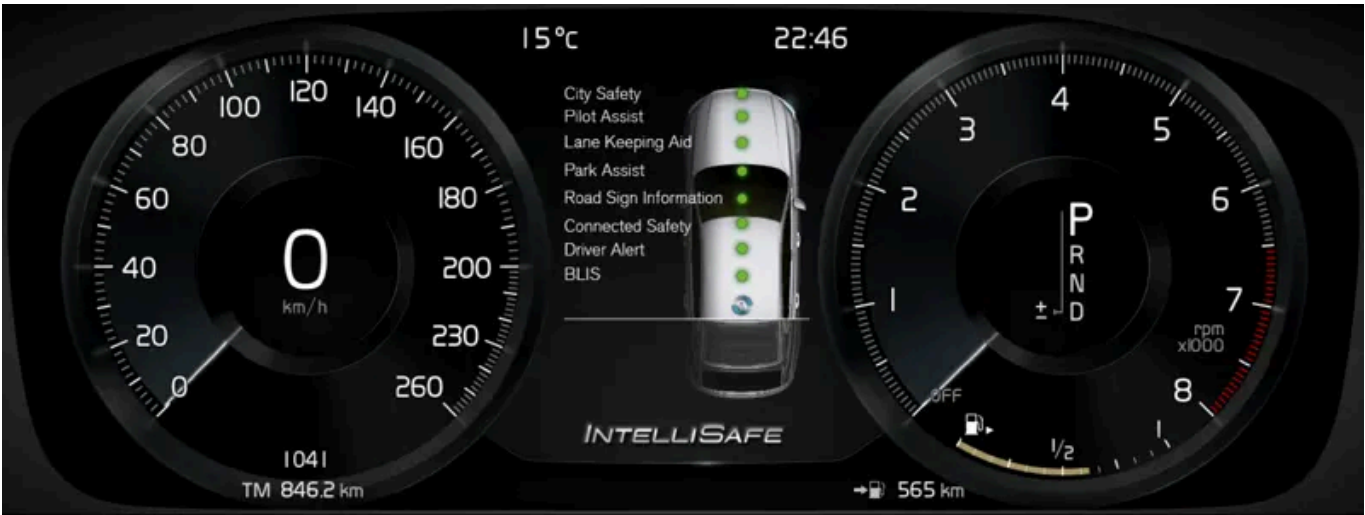
The illustration shows the 12" driver display
