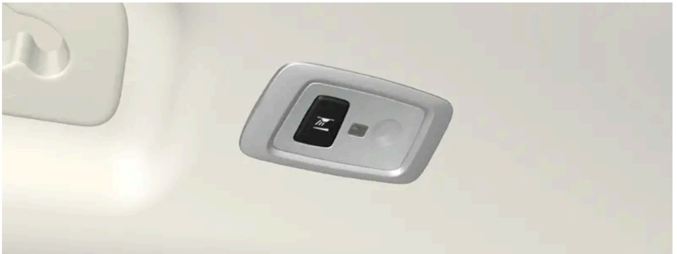
In cars with panoramic roof* there are two lamp units, one on each side of the roof.
