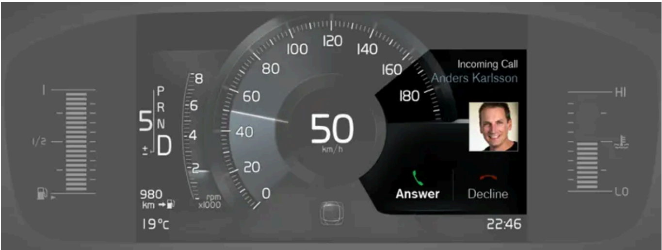
Example of message in the 8-inch driver display. The figure is schematic - parts may vary depending on car model.
