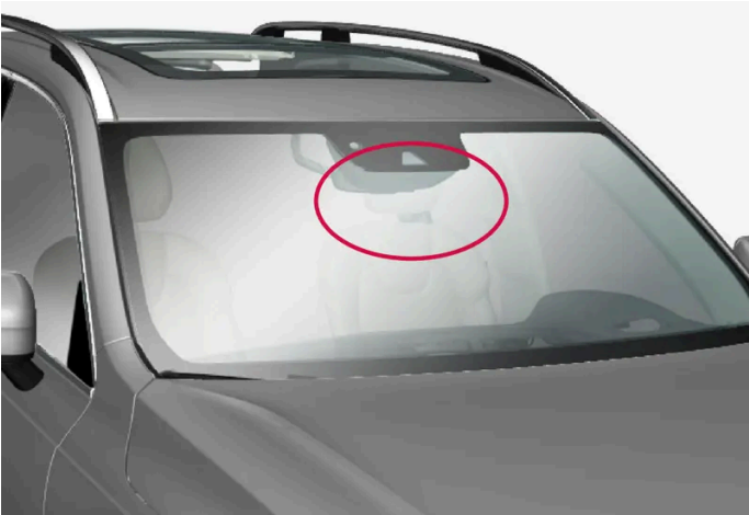
Location of front radar unit
