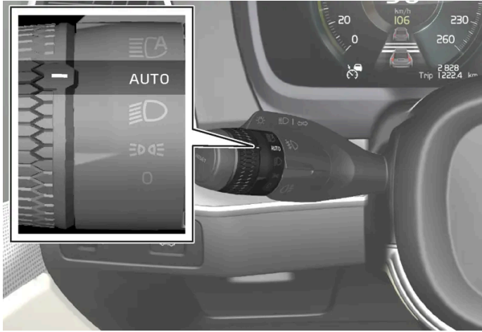
Stalk switch rotating ring in AUTO position.
