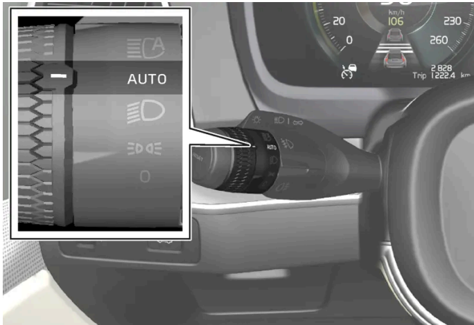
Stalk switch rotating ring in AUTO position.
