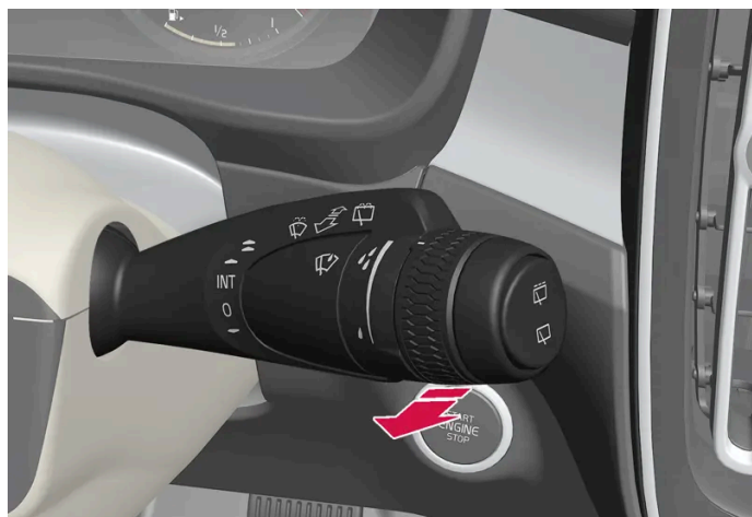
Washing function, right-hand stalk switch.
