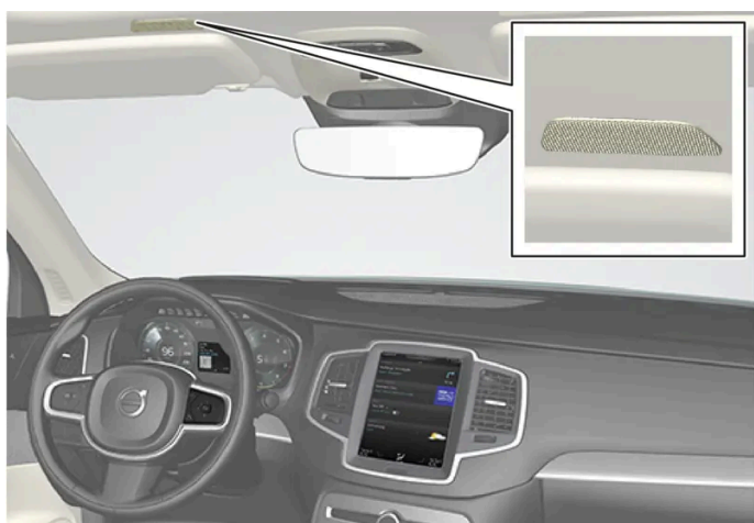
Voice control system microphone
