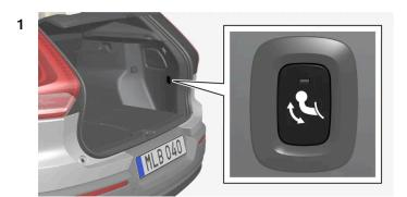
Open the tailgate. A button for extending/retracting the towbar is located on the right-hand side at the rear of the cargo area. An indicator lamp in the button must illuminate with a constant orange glow for the extension function to be active.
