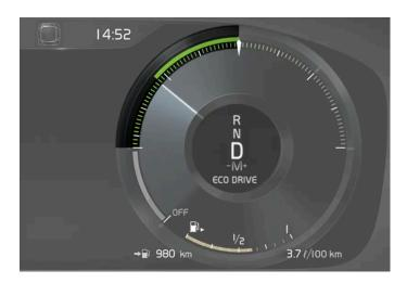
The ECO gauge indicates how fuel-efficient the driving is:
