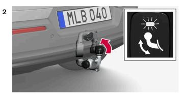
Lock the towbar by moving it back to its retracted position, where it is locked.
