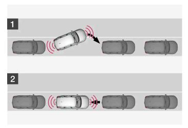
Principle for positioning during parallel parking.
