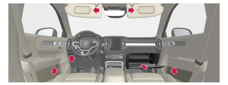
Storage compartment in door panel, card holder\* beside the steering wheel, sun visor and glovebox with extensible hook.
