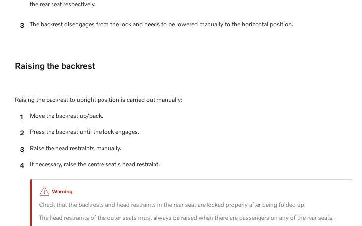
Pull the handles located on the car's left and right-hand backrests forwards to fold down the left and right-hand part of
