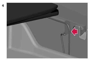
Carry on holding up the cargo area floor and press the lock spring on the other side as indicated by the arrow.
