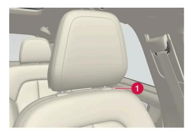
1 You can manually adjust the height of the head restraints by pressing in the button.
