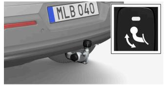
Move the towbar to its end position, where it is secured and locked in place - the indicator lamp illuminates with a constant orange glow.
