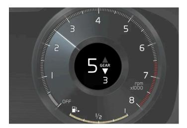
An up-arrow indicates a recommended change to a higher gear, and a down-arrow a recommended change to a lower gear.
