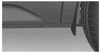
One of the car's four markings that show where the outer lifting points are located.
