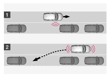
Principle for reversing into parallel parking.
