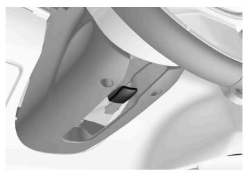
Lever for steering wheel adjustment.
