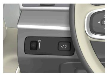
Thumbwheel (to left) for adjusting interior brightness.
