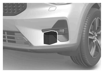
The support battery is located in the lower part of the engine compartment.
