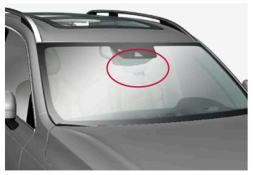
Location of front camera and radar unit
