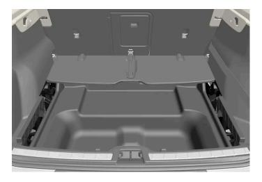
1 Lift the handle in the middle of the folding cargo area floor and fold it forwards.
