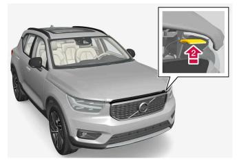
Move the handle under the bonnet upwards to release the catch and lift the bonnet.
