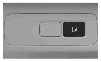
Turn off the car and open the fuel filler flap by pressing the fuel button  $\mathbb{B}$  on the dashboard, next to the steering wheel. 1
