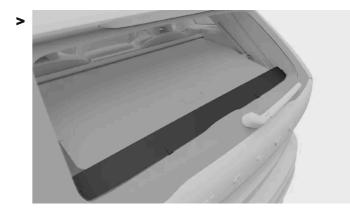
The boot hatch cover is installed and covers the boot storage compartment.
