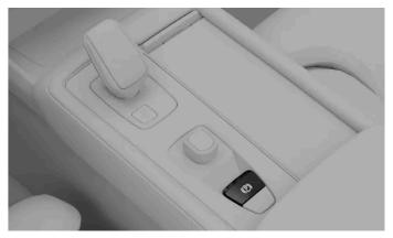
Manually engage the parking brake by pulling the parking brake switch.
