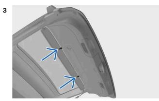
Push the two clips on the long side of the boot hatch cover upwards and click them into place on the boot hatch.
