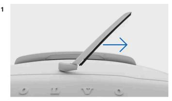
Grasp the centre of the wiper arm and lift it up and away from the rear windscreen. You may feel some resistance halfway – this is the lock position. You need to pull the wiper arm past the lock position so that it doesn't fall back onto the windscreen.
