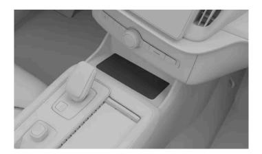
To use the wireless charger, your device should be certified to the Qi wireless charging standard. Also make sure that wireless charging is enabled on both the device<sup>[1]</sup> and on the charger itself. You can enable the charger in the centre display.
