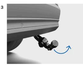
Manually pull the towbar to its end position.
