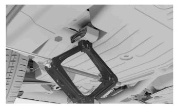
Raise the car to an appropriate height. Do not raise it higher than what's necessary for the work you're doing. 9
