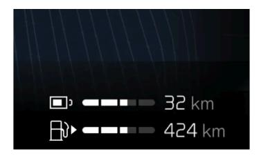
Your range is primarily related to your car's battery, the amount of fuel left in your car's tank and your driving practices but external conditions can also be a factor. The battery level and expected range are displayed in the driver display. The expected range is calculated based on your driving pattern, both current and historical.
