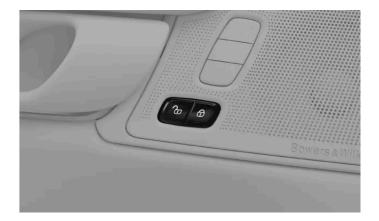
The central lock can be controlled from the front seats using the buttons on each respective door.
