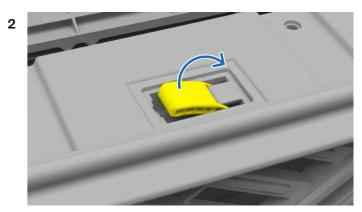
Locate the second lever below the front edge of the bonnet and pull it to the right.
