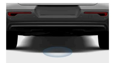
The sensor picks up movement under the rear bumper. Any detected movements unlock the boot.
