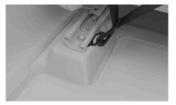
**4** Tighten the straps to make the safety net tight and more secure.
