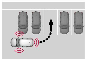
Principle for reversing into perpendicular parking.
