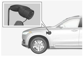
Charging cable handle and charging input socket.
