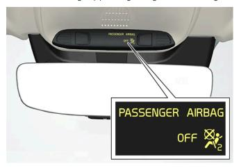
> A text message and a symbol in the roof console indicate that the airbag for the front passenger seat is deactivated.
