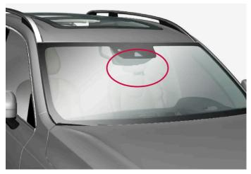
Location of front camera and radar unit
