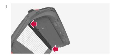
Turn the panel in the right direction with the screw side downward and guide the pin into the bracket on one side of the tailgate.
