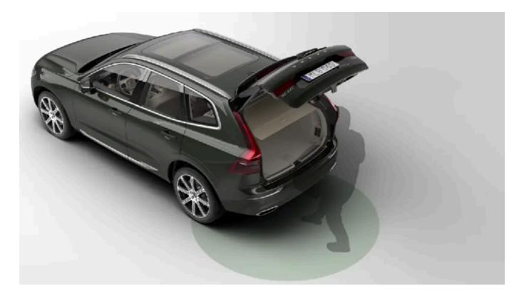
If the car is equipped with keyless locking and unlocking \* then you can unlock the tailgate with a foot movement.
