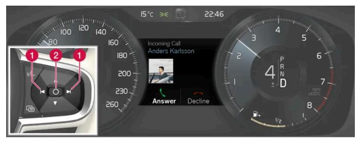
Examples of messages in the driver display and the steering wheel's right-hand keypad. The figure is schematic - parts may vary depending on car model.
