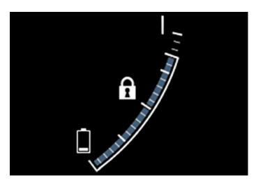
The symbol **1** is shown in the hybrid battery gauge when Hold is activated.
