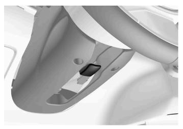
Lever for steering wheel adjustment.
