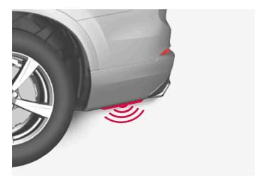
To activate opening or closing with a foot movement on a car equipped with skid plate, the kicking motion is made from the side of the car. One of the car's remote control keys must be within range (approx. 1 metre (3 feet)) for opening and closing to be possible.
