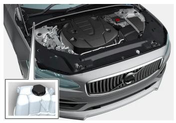
Coolant expansion tank, right-hand drive car
