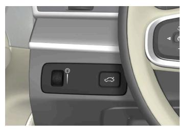
Thumbwheel (to left) for adjusting interior brightness.
