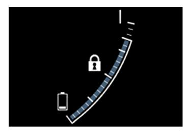
The firsymbol in the hybrid battery gauge indicates that the Hold function is activated, and the first symbol indicates that the Charge function is activated.
