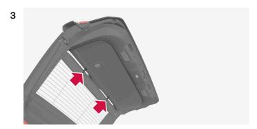
Press the two upper clips into the respective sockets in the tailgate so that they click into place.
