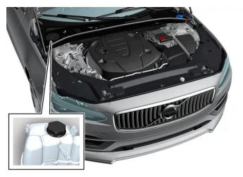
Coolant expansion tank, left-hand drive car
