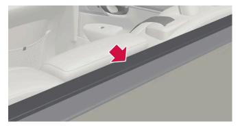
Ensure that the front panel is pointing down behind the backrests before the cassette is put in place.
