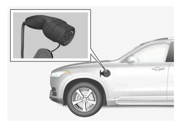
Charging cable handle and charging input socket.
