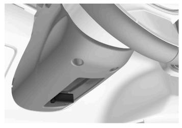
Lever for steering wheel adjustment.
