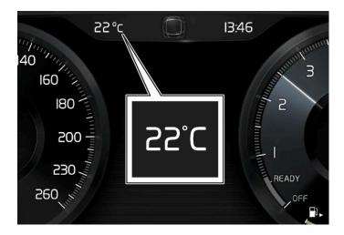
If the car has been stationary, the gauge may display a temperature reading that is too high.
