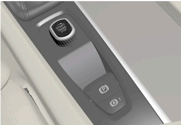
Start knob in the tunnel console.
