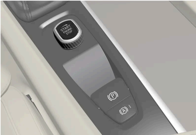
Start knob in the tunnel console.
