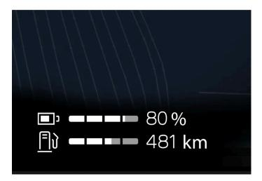
The battery gauge in the lower part of the driver display shows the State of Charge (SoC) for the battery as well as range to empty battery.
