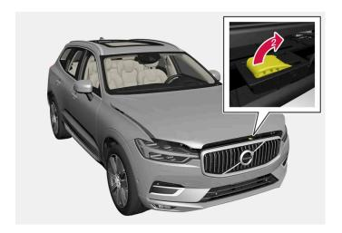
😰 Sweep from left to right in the opening under the bonnet, move the handle up and to the side to release catch and lift the bonnet.
