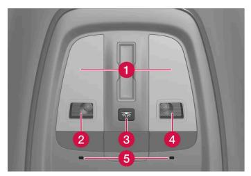
Lighting and controls in the roof console.
