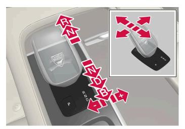
Overview of gear lever and gear positions.
