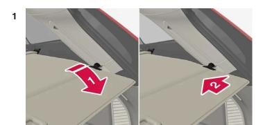
Grip the handle and pull the cargo cover out to the end position.
