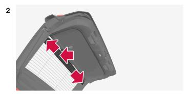
Carefully pull the panel away from the bracket on one side of the tailgate, and then from the other side. If necessary, clamp the panel slightly so that it is more flexible and to facilitate removal.
