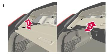
Press the cargo cover's handle section upwards slightly.
