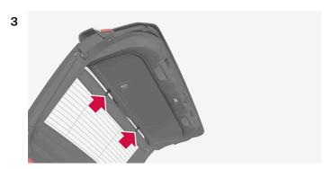
Press the two upper clips into the respective sockets in the tailgate so that they click into place.
