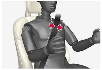
The seatbelt must pass over the shoulder (not down over the arm).
