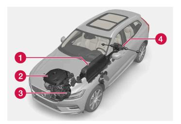
1 Hybrid battery - The function of the hybrid battery is to store energy. It receives energy when charging from the mains power circuit, during regenerative braking or from the high-voltage generator. It provides energy for electric operation as well as for temporarily operating the electric air conditioning during the preconditioning of the passenger compartment.
