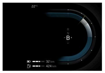
Gear shift indicator in the driver display.
