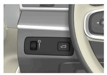
Thumbwheel (to left) for adjusting interior brightness.
