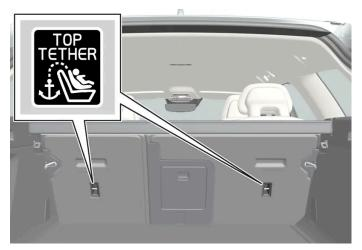
Mounting point locations for the rear seat are indicated by symbols on the rear of the backrest.
