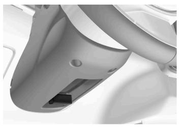
Lever for steering wheel adjustment.
