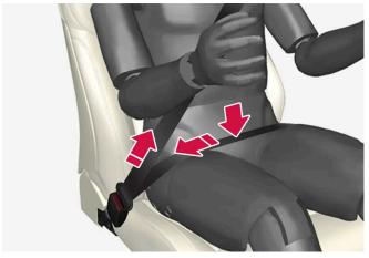
The hip strap must be positioned low down (not over the abdomen).
