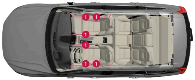
Location of adjustable air vents in the passenger compartment.
