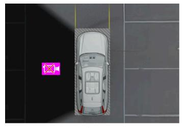
Example for showing when the car's left camera is non-operational.  $\label{eq:cample_show}$
