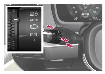
Steering wheel stalk switch with rotating ring.
