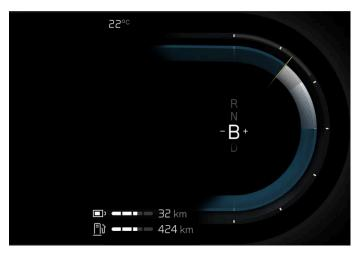
Gear shift indicator in the driver display.
