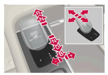
Overview of gear lever and gear positions.
