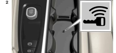
Place the key on the key symbol in the backup reader in the tunnel console's cup holder.
