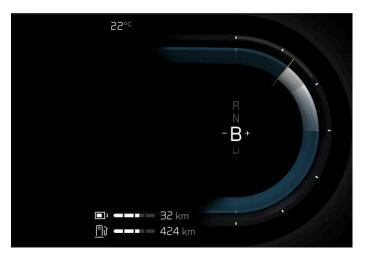
Gear shift indicator in the driver display.
