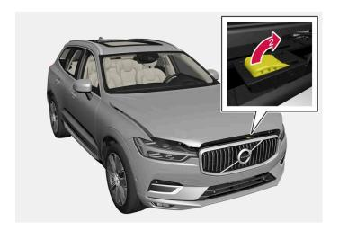
😰 Sweep from left to right in the opening under the bonnet, move the handle up and to the side to release the bonnet from the bonnet lock's catch and lift the bonnet.
