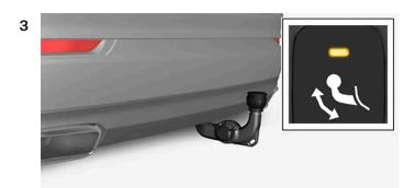
Move the towbar to its end position, where it is secured and locked in place - the indicator lamp illuminates with a constant orange glow.
