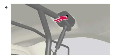
Insert the supplied screw and tighten using the supplied 6 mm Allen key. Repeat on the other side. Recommended tightening torque: 20 Nm (15 foot-pounds).
