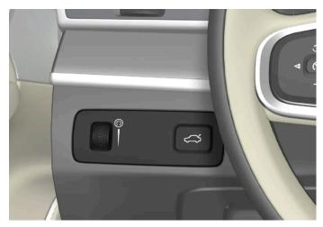
Thumbwheel (to left) for adjusting interior brightness.
