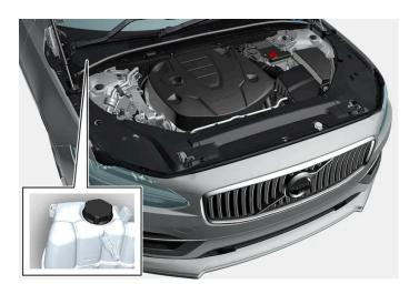
Coolant expansion tank, right-hand drive car.
