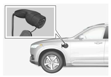
Charging cable handle and charging input socket.
