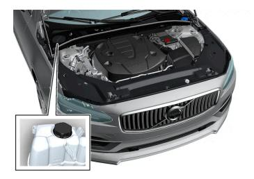
Coolant expansion tank, left-hand drive car.
