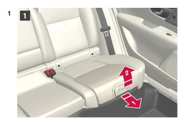
Pull the handle forwards and upwards to release the seat cushion.
