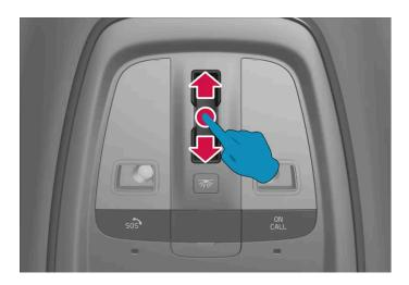
Make a smooth and continuous swiping motion backwards/forwards over the touch-sensitive control to fully open/close the panoramic roof. In the event of problems, try moving more quickly or more slowly.
