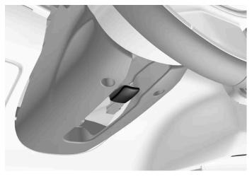
Lever for steering wheel adjustment.
