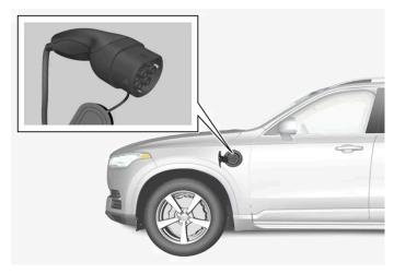
Charging cable handle and charging input socket.
