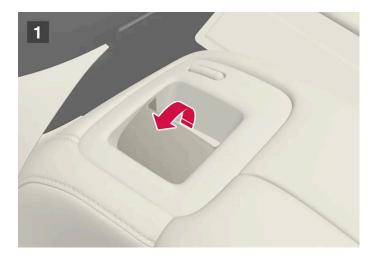
For cars with electronically controlled head restraint folding\*, the outer head restraints can be folded using handles on the top of the seat, see figure 1. Note that this method also folds the backrests. If only the head restraints shall be folded, e.g. to improve visibility, it can be performed from the centre display instead\*.
