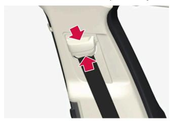
Press together the seat mounting and move the seatbelt up or down.
