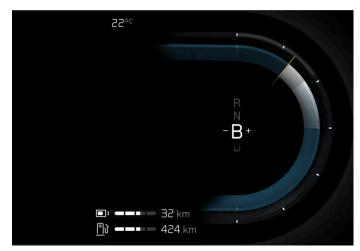
Gear shift indicator in the driver display.
