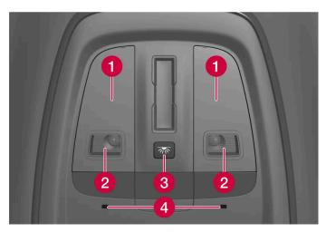
Lighting and controls in the roof console.
