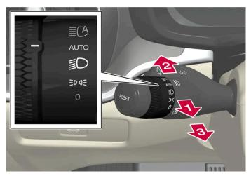
Steering wheel stalk switch with rotating ring.
