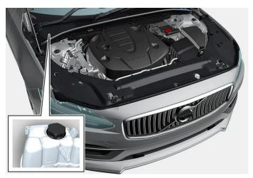
Coolant expansion tank, right-hand drive car.
