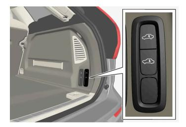
Use the buttons in the cargo area to regulate the height of the car's rear section and facilitate loading and unloading or when connecting or disconnecting a trailer.
