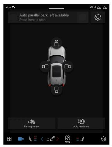
Camera view shows the park assist cameras (PAC<sup>[1]</sup>), which displays a composite 360° view and separate views for each of the four cameras: rear, front, left or right camera view.
