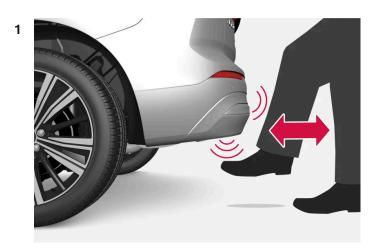
Make **one** forward kicking motion in the sensor area under the rear bumper. Then take a step back. The bumper must not be touched.
