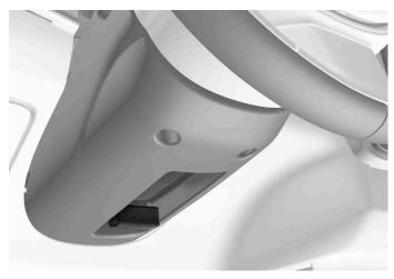
Lever for steering wheel adjustment.
