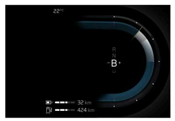
Gear shift indicator in the driver display.
