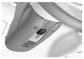
Lever for steering wheel adjustment.
