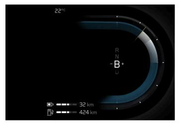
Gear shift indicator in the driver display.
