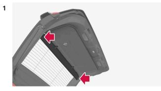
Turn the panel in the right direction with the screw side downward and guide the pin into the bracket on one side of the tailgate.
