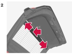
Carefully pull the panel away from the bracket on one side of the tailgate, and then from the other side. If necessary, clamp the panel slightly so that it is more flexible and to facilitate removal.
