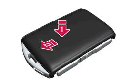
Refit the rear shell in reverse order to how it was removed. There is no logotype on the rear shell. Press in the shell until you hear a click, and then slide it the last few millimetres to its original position.
