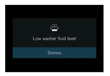
Messages are shown in the middle of the driver display. The composition may vary and is shown together with graphics, symbols or buttons for acknowledging the message or accepting a request, for example.
