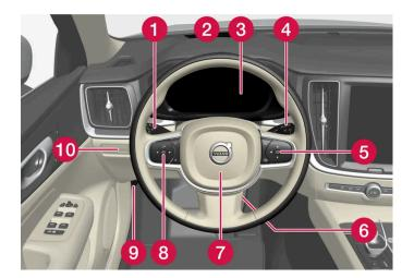
1 Position lamps, daytime running lights, dipped beam, main beam, direction indicators, rear fog lamp, resetting the trip meter
