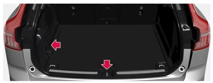
Cargo area with mesh pocket\* or side panel, and storage space under the cargo area floor.
