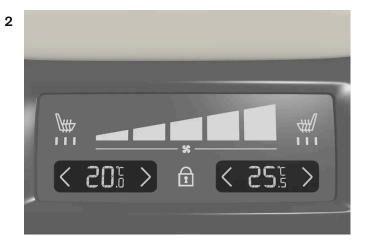
1 Press the unlocking button on the tunnel console climate panel to access the controls.
