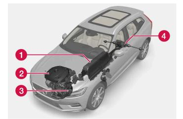
🚺 Hybrid battery - The function of the hybrid battery is to store energy. It receives energy when charging from the mains power circuit, during regenerative braking or from the high-voltage generator. It provides energy for electric operation as well as for temporarily operating the electric air conditioning during the preconditioning of the passenger compartment.
