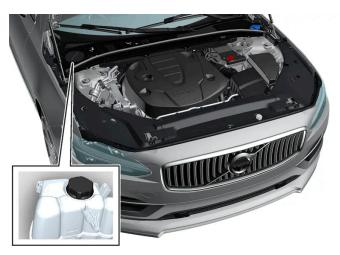
Coolant expansion tank, left-hand drive car.
