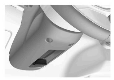
Lever for steering wheel adjustment.
