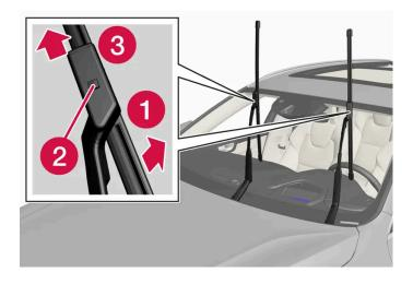
Fold up the wiper arm when it is in service position. Service position is activated/deactivated via the centre display when the car is stationary and the windscreen wipers are not switched on.
