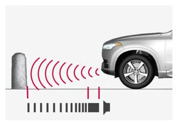
The warning signal has a constant acoustic signal at less than approx. 30 cm (1 foot) from an obstacle.
