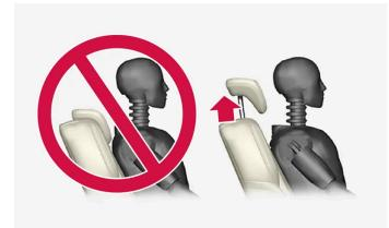
The centre seat's head restraint must be adjusted according to the passenger's height so that, if possible, the whole of the back of the head is covered. Slide it up manually as required.
