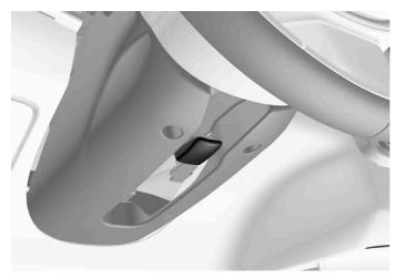
Lever for steering wheel adjustment.
