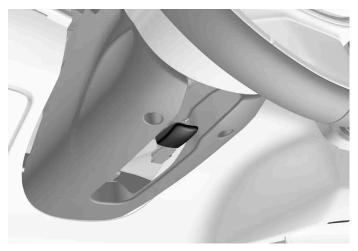
Lever for steering wheel adjustment.
