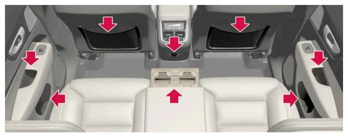
Storage compartment in the door panel, cup holder\* in the centre seat backrest, storage pocket on the front seat backrest, and USB ports in the tunnel console.
