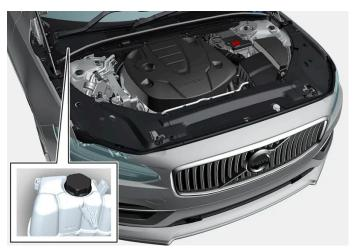
Coolant expansion tank, right-hand drive car.
