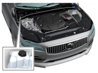
Coolant expansion tank, left-hand drive car.
