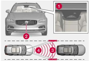
The camera and radar units measure the distance to the vehicle ahead and detect lane markings.
