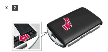
Slide the catch that was behind the front shell to the side, and slide the rear shell away from the key ring bracket.
