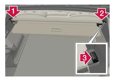
Insert one of the cargo cover's end pieces in the recess in the side panel in the cargo area.
