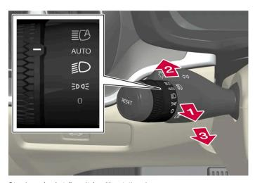
Steering wheel stalk switch with rotating ring.
