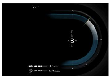
Gear shift indicator in the driver display.
