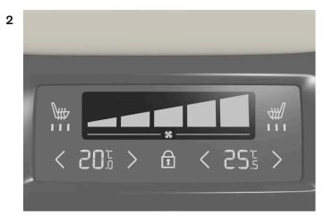
Fan controls on the climate panel at the rear of the tunnel console.
