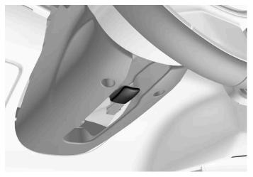
Lever for steering wheel adjustment.
