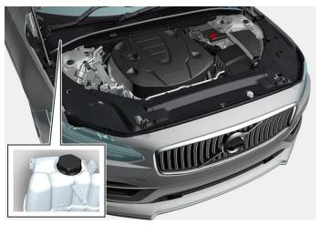
Coolant expansion tank, right-hand drive car.
