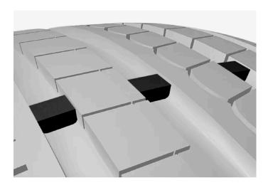
A tread wear indicator is a narrow elevation across the longitudinal grooves of the tyre's tread pattern. On the side of the tyre are the letters TWI (Tread Wear Indicator). When the tyre's tread depth is down to 1.6 mm (1/16 inch), the tread will be level in height with the tread wear indicators. Change to new tyres as soon as possible. Remember that tyres with little tread depth provide very poor grip in rain and snow.
