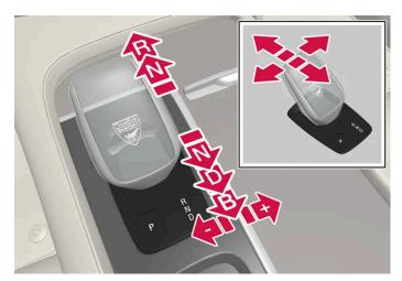
Overview of gear lever and gear positions.
