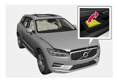
2 Sweep from left to right in the opening under the bonnet, move the handle up and to the side to release catch and lift the bonnet.
