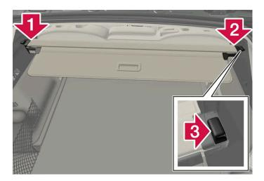
Insert one of the cargo cover's end pieces in the recess in the side panel in the cargo area.
