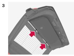
Press the two upper clips into the respective sockets in the tailgate so that they click into place.
