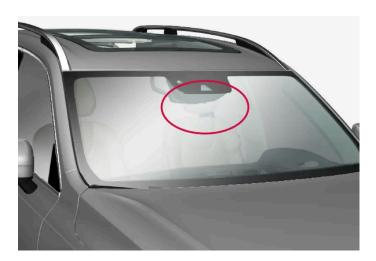
Location of front camera and radar unit
