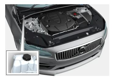
Coolant expansion tank, right-hand drive car
