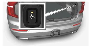
Open the tailgate. A button for extending/retracting the towbar is located on the right-hand side at the rear of the cargo area. An indicator lamp in the button must illuminate with a constant orange glow for the extension function to be active.
