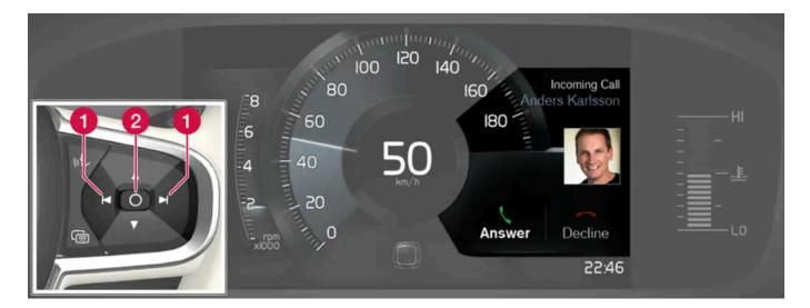
Examples of messages in the driver display<sup>[1]</sup> and the steering wheel's right-hand keypad. The figure is schematic - parts may vary depending on car model.
