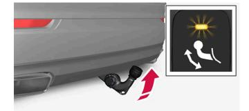
> The towbar extends out and down in an unlocked position - the indicator lamp flashes orange. The tow hook is ready to continue moving to the locked position.
