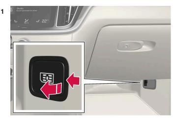
Fit a personal SIM card into the holder by the floor on the passenger side. Note that a **mini SIM** is required to fit the car's card reader.
