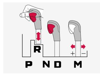
Gear selector inhibitor for cars with the large gear lever.
