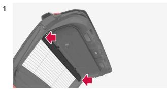
Turn the panel in the right direction with the screw side downward and guide the pin into the bracket on one side of the tailgate.
