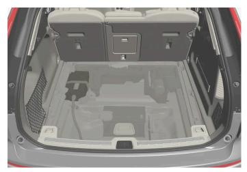
If the car is the mild hybrid type, it will have a 48 V support battery instead, located on the left of the cargo area. The 48 V support battery must only be handled by an authorised workshop.
