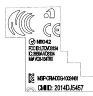
CEM marking for the remote control key system. For supplementary type approval numbers, see following tables.
