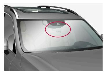
Location of front camera and radar unit
