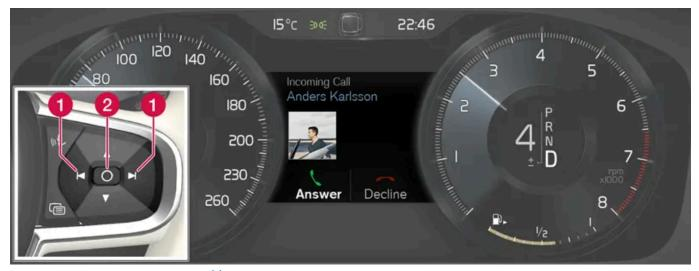
Examples of messages in the driver display<sup>[2]</sup> and the steering wheel's right-hand keypad. The figure is schematic - parts may vary depending on car model.
