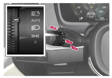
Steering wheel stalk switch with rotating ring.
