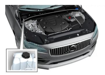
Coolant expansion tank, left-hand drive car
