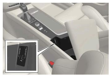
USB ports (type A) in the tunnel console. Allow the cable to lie forwards so that it is not trapped when the lid is closed.
