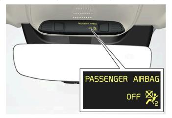
> A text message and a symbol in the roof console indicate that the airbag for the front passenger seat is deactivated.
