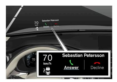
The head-up display shows warnings and information relating to speed, cruise control functions, navigation, etc. in the driver's field of vision. Road Sign Information and incoming phone calls can also be shown in the head up display.
