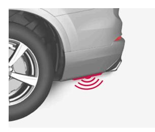
To activate opening or closing with a foot movement on a car equipped with skid plate, the kicking motion is made from the side of the car. One of the car's remote control keys must be within range (approx. 1 metre (3 feet)) for opening and closing to be possible.
