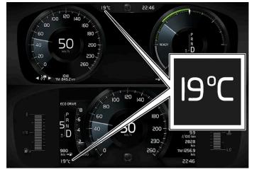
Outside temperature gauge location in the 12-inch\* and 8-inch driver display. The figure is schematic - parts may vary depending on car model.
