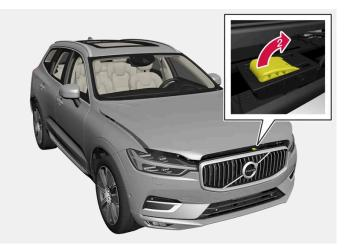
😰 Sweep from left to right in the opening under the bonnet, move the handle up and to the side to release the bonnet from the bonnet lock's catch and lift the bonnet.
