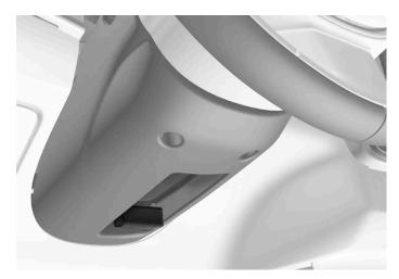
Lever for steering wheel adjustment.
