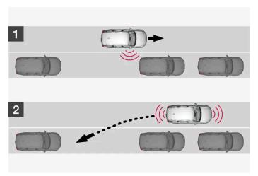
Principle for reversing into parallel parking.
