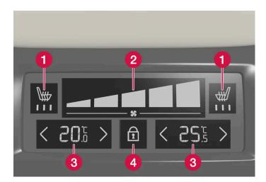
1 Controls for heated rear seat\*.
