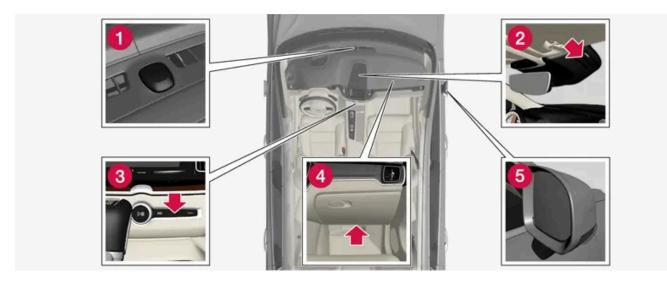
**1** Sun sensor - on the upper side of the instrument panel.
