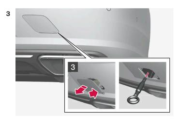
> The cover pivots around its centre line and can then be removed.
