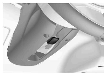
Lever for steering wheel adjustment.
