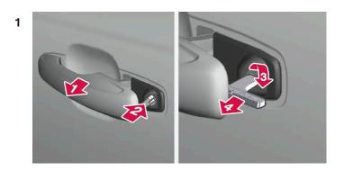
Pull out the front door's handle on the left-hand side of the car to its end position.<sup>[1]</sup>
