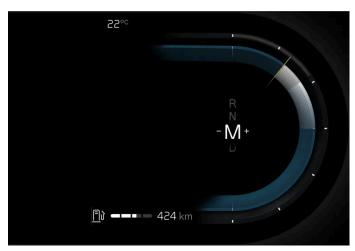
Gear shift indicator in the driver display.
