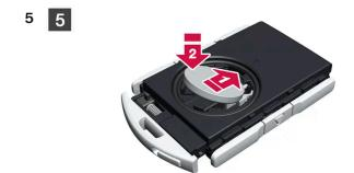
Install a new battery with the (+) side up. Avoid touching the key's battery contacts with your fingers.
