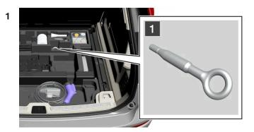
1 Take out the towing eye from the foam block under the floor in the cargo area.
