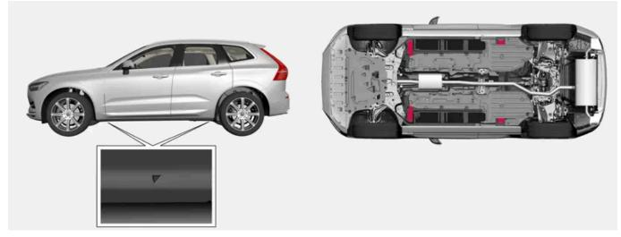
The triangles in the plastic cover indicate the locations of the lifting points (marked in red).
