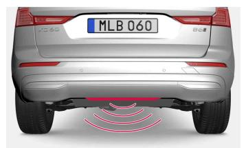
The sensor is located in the centre of the bumper.
