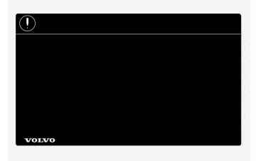
White ISO symbols and white text/image on black or blue warning field and message field. Used to indicate the presence of danger which, if the warning is ignored, may result in damage to property.
