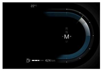
Gear shift indicator in the driver display.
