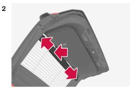
Carefully pull the panel away from the bracket on one side of the tailgate, and then from the other side. If necessary, clamp the panel slightly so that it is more flexible and to facilitate removal.
