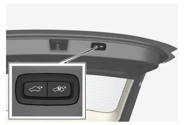
Location of the button/buttons on the underside of the tailgate.
