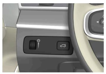
Thumbwheel (to left) for adjusting interior brightness.
