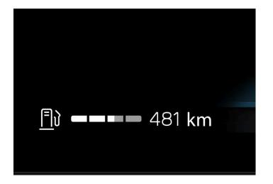
The white zone in the fuel gauge indicates the quantity of fuel in the tank.
