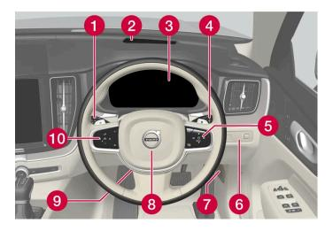
1 Position lamps, daytime running lights, dipped beam, main beam, direction indicators, front fog lamps/cornering lights\*, rear fog lamp, resetting the trip meter
