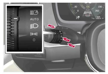
Steering wheel stalk switch with rotating ring.
