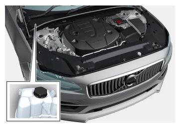
Coolant expansion tank, right-hand drive car.
