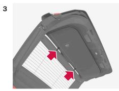
Press the two upper clips into the respective sockets in the tailgate so that they click into place.
