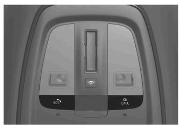
The functions are available via the ON CALL and SOS buttons in the car's roof.
