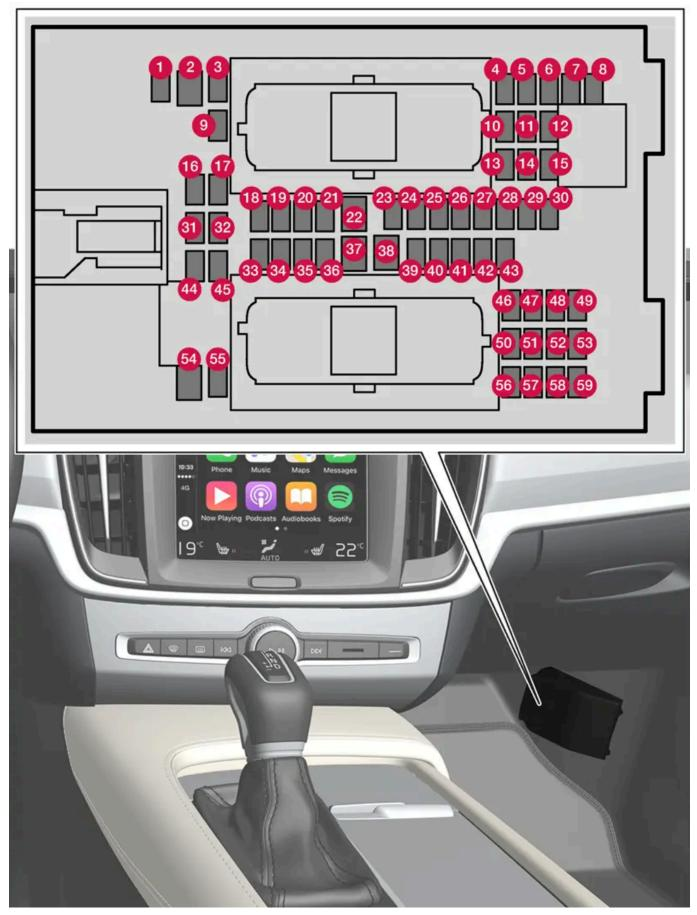
The fuse box is located behind the floor mat/side panel.
