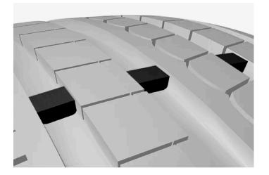
A tread wear indicator is a narrow elevation across the longitudinal grooves of the tyre's tread pattern. On the side of the tyre are the letters TWI (Tread Wear Indicator). When the tyre's tread depth is down to 1.6 mm (1/16 inch), the tread will be level in height with the tread wear indicators. Change to new tyres as soon as possible. Remember that tyres with little tread depth provide very poor grip in rain and snow.
