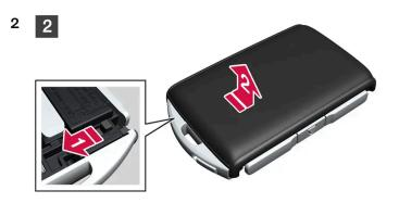
Slide the catch that was behind the front shell to the side, and slide the rear shell away from the key ring bracket.
