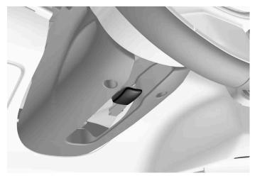
Lever for steering wheel adjustment.
