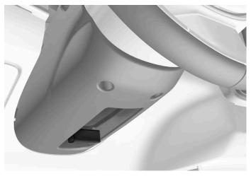
Lever for steering wheel adjustment.
