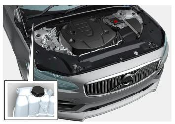
Coolant expansion tank, right-hand drive car.
