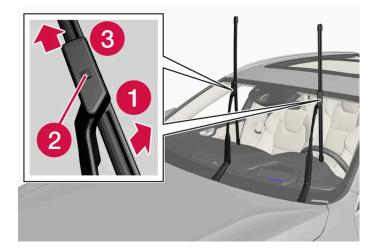
Fold up the wiper arm when it is in service position. Service position is activated/deactivated via the centre display when the car is stationary and the windscreen wipers are not switched on.
