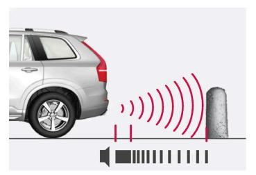
The warning signal has a constant tone at less than approx. 30 cm (1 foot) from an obstacle.
