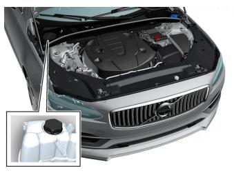
Coolant expansion tank, left-hand drive car.
