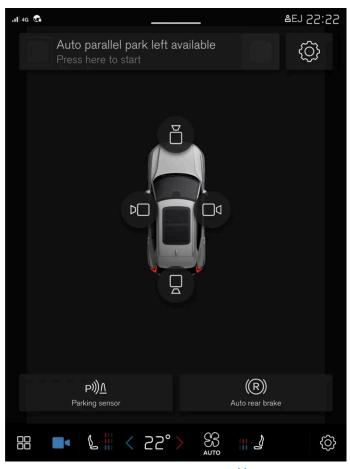
Camera view shows the park assist cameras (PAC $^{[1]}$ ), which displays a composite 360° view and separate views for each of the four cameras: rear, front, left or right camera view.
