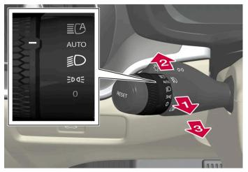
Steering wheel stalk switch with rotating ring.
