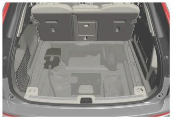
Cars of the mild hybrid type have a 48 V support battery under the cargo area. The battery must only be handled by an authorised workshop.
