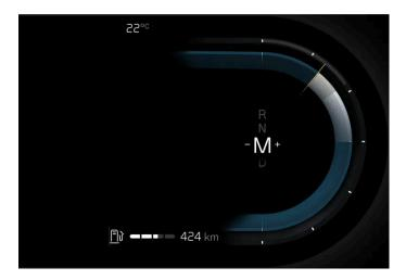
In M position, it is possible to change gear manually. The car engine-brakes when the accelerator pedal is released.
