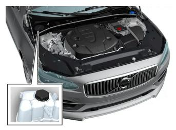
Coolant expansion tank, left-hand drive car.
