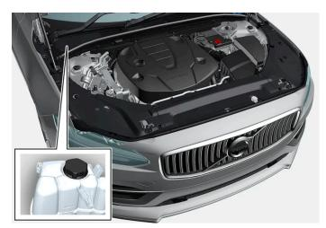
Coolant expansion tank, right-hand drive car.
