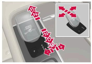
Overview of gear lever and gear positions.
