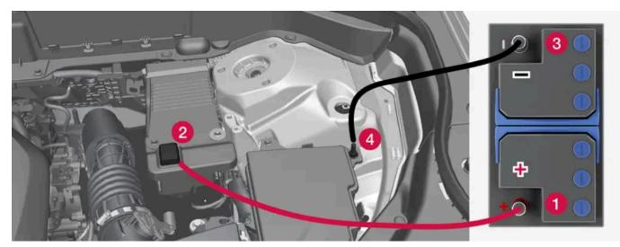
Charging points for jump starting own car. The appearance in the engine compartment may vary depending on car model and equipment level.
