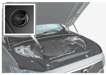
In some cases, oil may need to be topped up between service intervals. No action with regard to engine oil level needs to be taken until a message is shown in the driver display.
