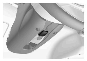
Lever for steering wheel adjustment.
