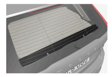
A panel must be fitted on the tailgate when using the cargo cover.
