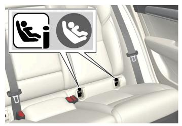
Mounting point locations for the rear seat are indicated by symbols<sup>[1]</sup> on the covers that conceal the mounting points.
