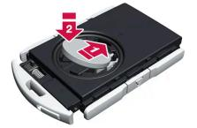
Install a new battery with the (+) side up. Avoid touching the key's battery contacts with your fingers.
