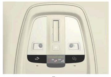
The functions are available via the  $\mathcal{R}$  and SOS buttons in the car's roof.
