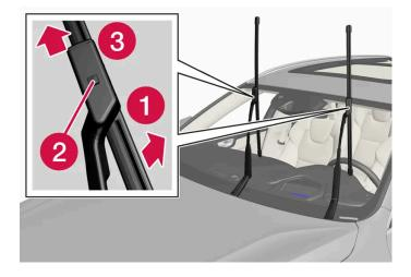
Make sure that the windscreen wipers are in service position and fold up the wiper arms. Service position is activated/deactivated via the centre display when the car is stationary and the windscreen wipers are not switched on.
