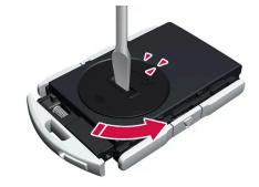
Turn the battery cover anticlockwise to OPEN position. Use a screwdriver or a coin, for example.
