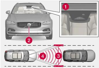
The camera and radar units measure the distance to the vehicle ahead and detect lane markings.
