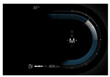
Gear shift indicator in the driver display.
