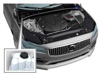
Coolant expansion tank, left-hand drive car.
