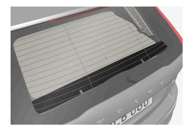
A panel must be fitted on the tailgate when using the cargo cover.
