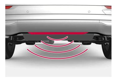
The sensor is located in the centre of the bumper.
