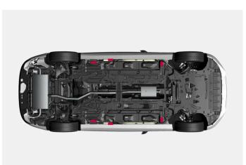
The car has outer lifting points for low level lifting, and inner lifting points for high level lifting, such as garage jack or lifting arms.
