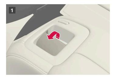
For cars with electronically controlled head restraint folding\*, the outer head restraints can be folded using handles on the top of the seat, see figure **1**. Note that this method also folds the backrests. If only the head restraints shall be folded, e.g. to improve visibility, it can be performed from the centre display instead\*.
