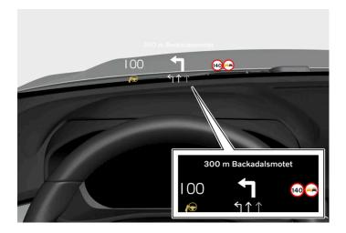
The head-up display projects information from the driver display onto the windscreen in front of the driver. The information can only be seen from the driver's position.
