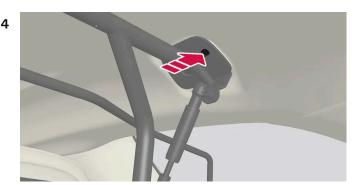
Insert the supplied screw and tighten using the supplied 6 mm Allen key. Repeat on the other side. Recommended tightening torque: 20 Nm (15 foot-pounds).
