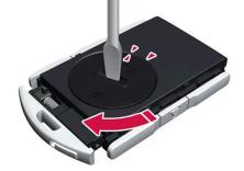
Refit the battery cover and turn clockwise to CLOSE position.
