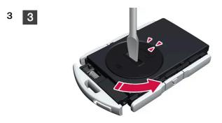
Turn the battery cover anticlockwise to OPEN position. Use a screwdriver or a coin, for example. Lift off the battery cover. If it is difficult to detach, you can prize it upward using a narrow tool.
