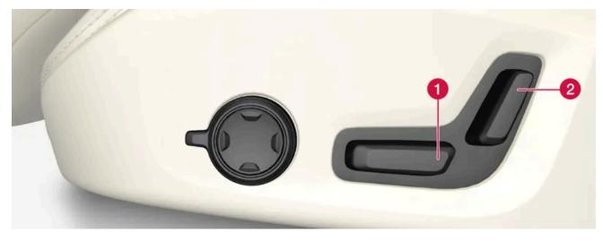
**1** Move the passenger seat forward/backward by adjusting the control forward/backward.
