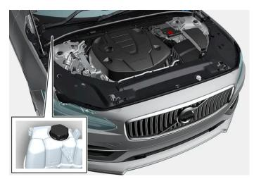
Coolant expansion tank, right-hand drive car.
