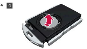
The battery (+) side is facing upwards. Loosen the battery by pressing on its edge and then lifting it out.
