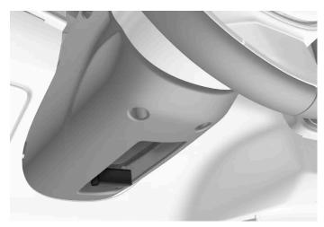
Lever for steering wheel adjustment.
