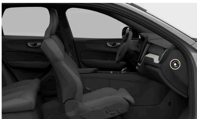
Location of the passenger airbag switch
