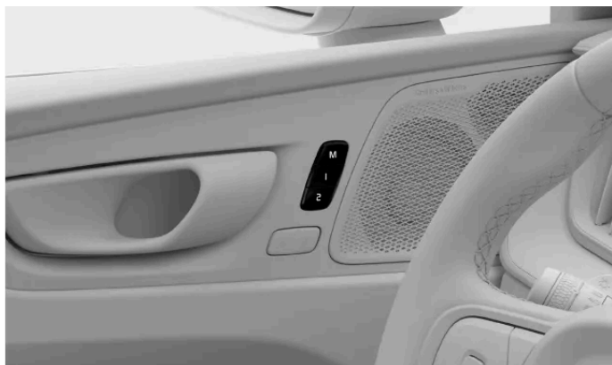
Location of the preset seat adjustment buttons
