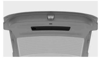
The warning triangle is located on the inside of the boot hatch. Open the compartment by turning the handle so that it's vertical and then pulling it.
