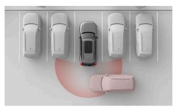
Your car can detect a car crossing behind you, for example when reversing out of a parking spot. This allows it to warn you so that you can slow down or brake.
