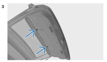
Push the two clips on the long side of the boot hatch cover upwards and click them into place on the boot hatch.
