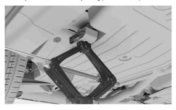
g Raise the car to an appropriate height. Do not raise it higher than what's necessary for the work you're doing.
