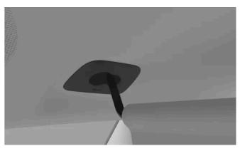
Fasten the lower corners of the net to the load-retaining eyelets behind the seats.
