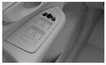
Controls for adjusting the wing mirrors
