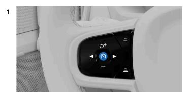
When it's safe to do so, press the Pilot Assist button ( on the steering wheel.
