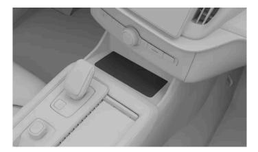
To use the wireless charger, your device should be certified to the Qi wireless charging standard. Also make sure that wireless charging is enabled on both the device [1] and on the charger itself. You can enable the charger in the centre display.
