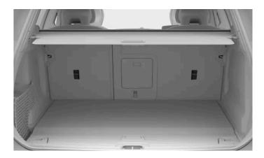
The top tether anchorage point locations for the rear seats are indicated by the top tether symbol.
