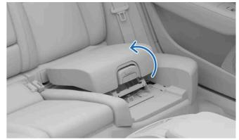
Lift the child seat upwards by the front end and push it back against the backrest.
