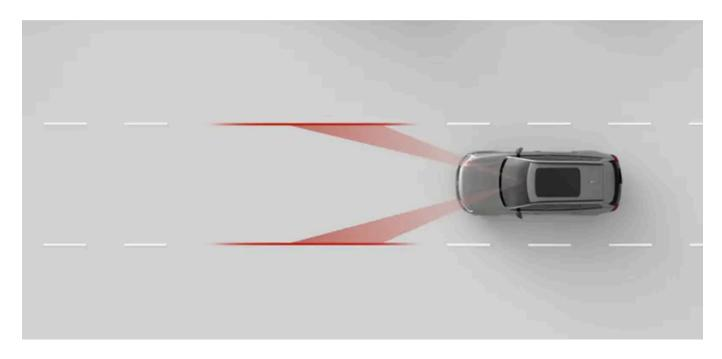
When lane keeping aid is enabled, the car can alert you if you are about to drift out of your lane and it can ask you to steer the car with attention. It can also perform steering interventions. Lane keeping aid relies on the car's forward-facing camera to identify road markings and your position in the lane.
