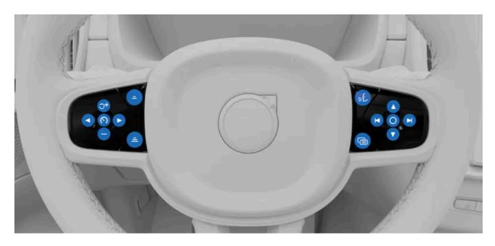
The buttons on your steering wheel's left-hand side control driver support features.
