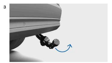
Manually pull the towbar to its end position.
