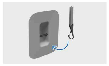
Fastening tether to top tether anchorage point
