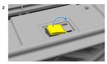
Locate the second lever below the front edge of the bonnet and pull it to the right.
