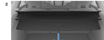
Pull the load cover screen by the handle over the boot's side panels.
