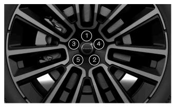
Tighten the wheel fasteners crosswise.
