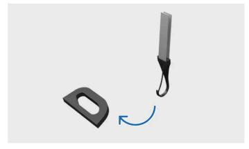
Fastening tether to lower tether anchorage point
