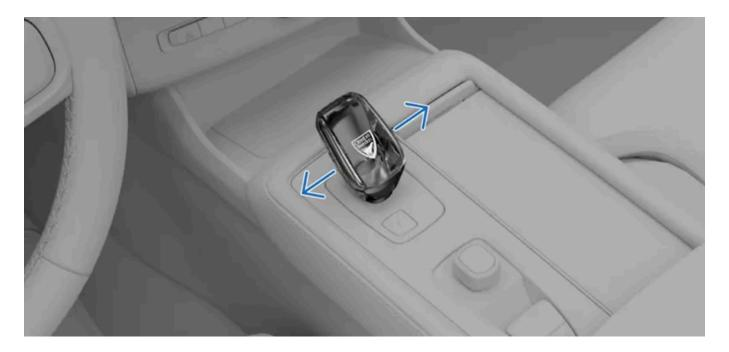
After selecting gear M, you can manually shift gears by moving the gear selector to the left or right.
