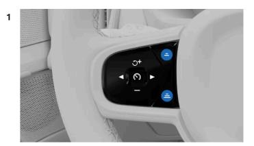
Adjust the time interval to vehicles ahead using the buttons on the steering wheel.
