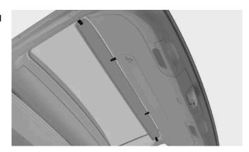
Guide one of the pins on the boot hatch cover into the bracket on one side of the boot hatch.
